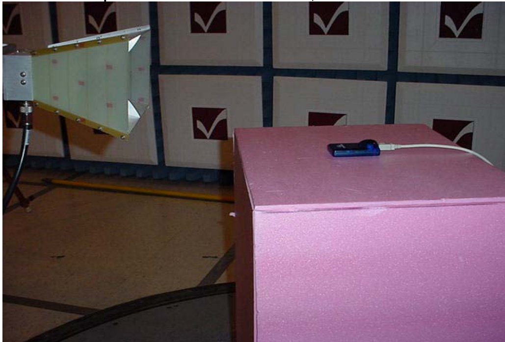
Setup for the Radiated Emissions Test; 0.3 Meter Distance
