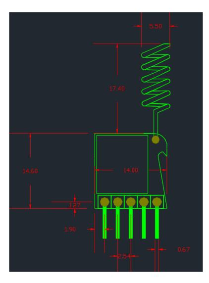
RYLR998 868/915MHz Lora Antenna Transceiver Module **REYAX**
