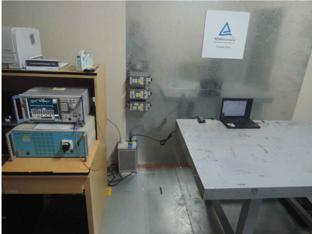
Photograph 11: Set-up for Mains Conducted testing Back
