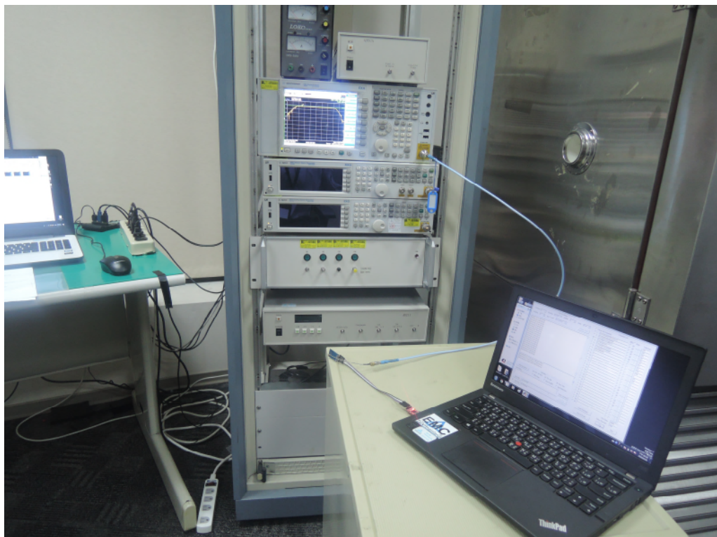
Photograph 7: Set-up for Conducted testing
