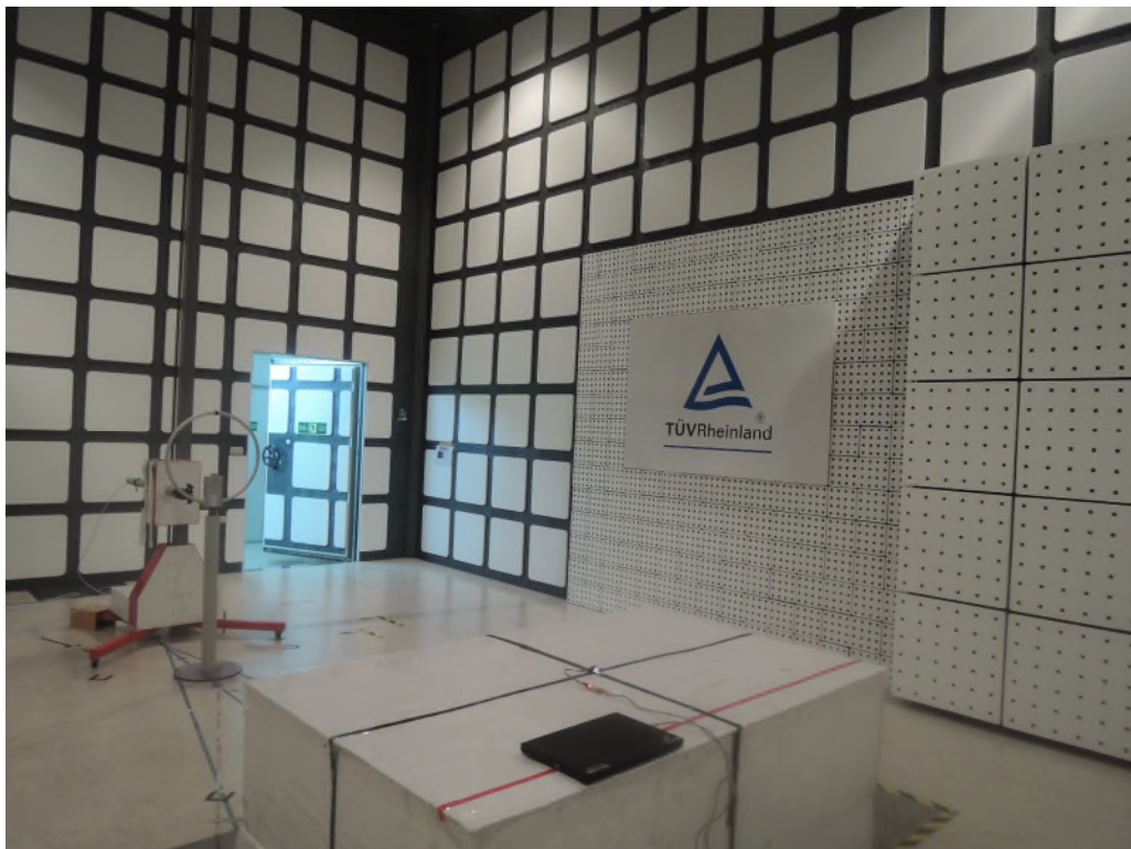
Photograph 5: Set-up for Spurious Emissions (Back View 3)
