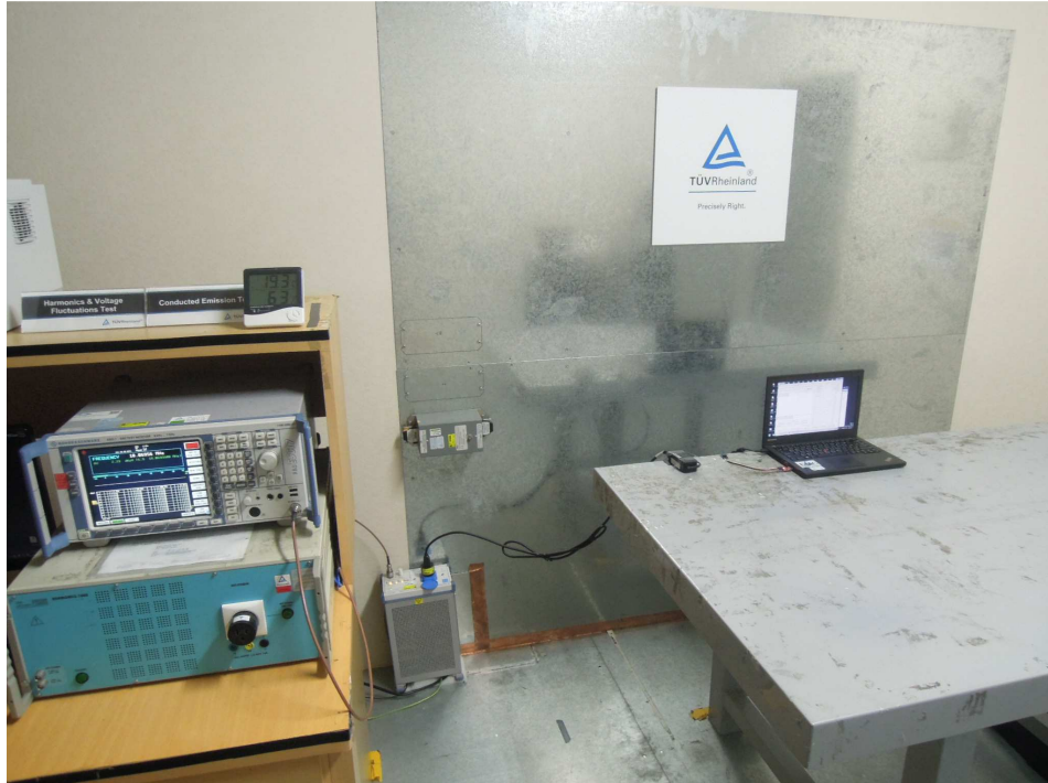
Photograph 6: Set-up for for Mains Conducted testing Front
