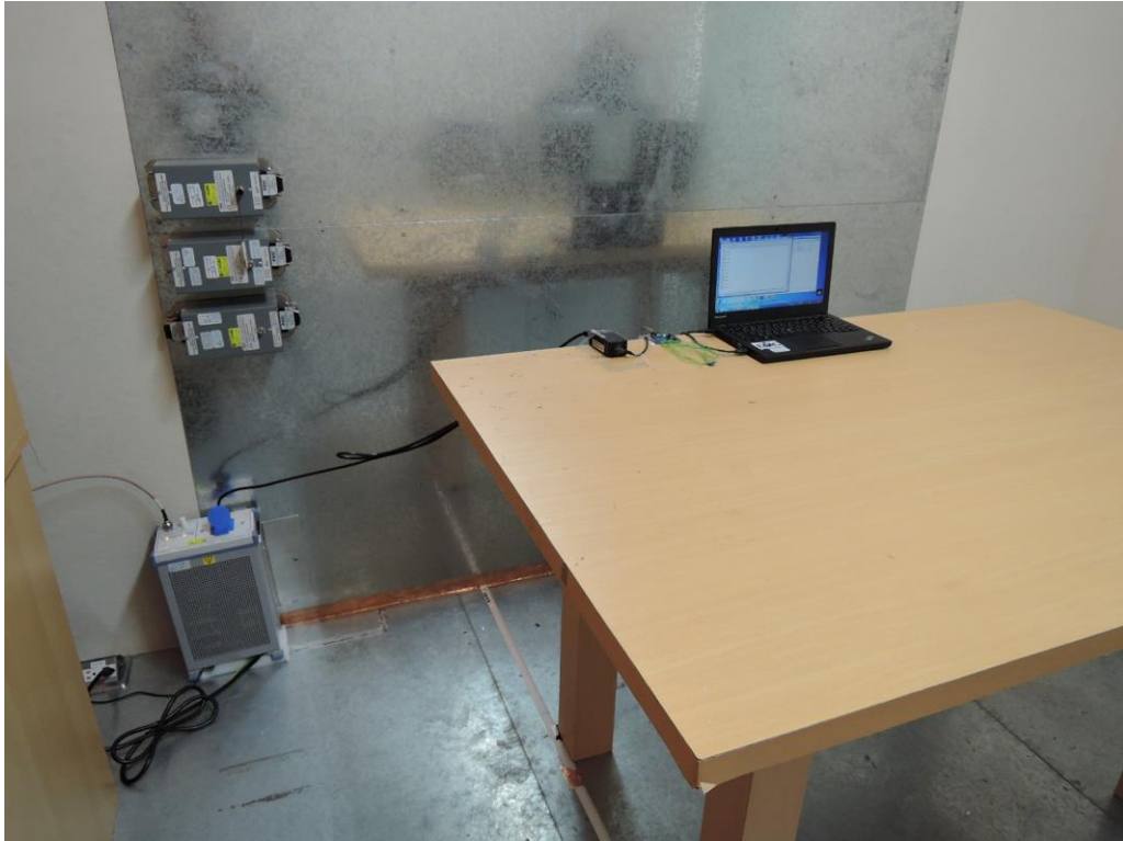
Photograph 6: Set-up for for Mains Conducted testing Front
