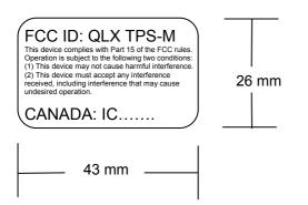
Label for DSS-Modul. It will be placed on the backside of the module.
