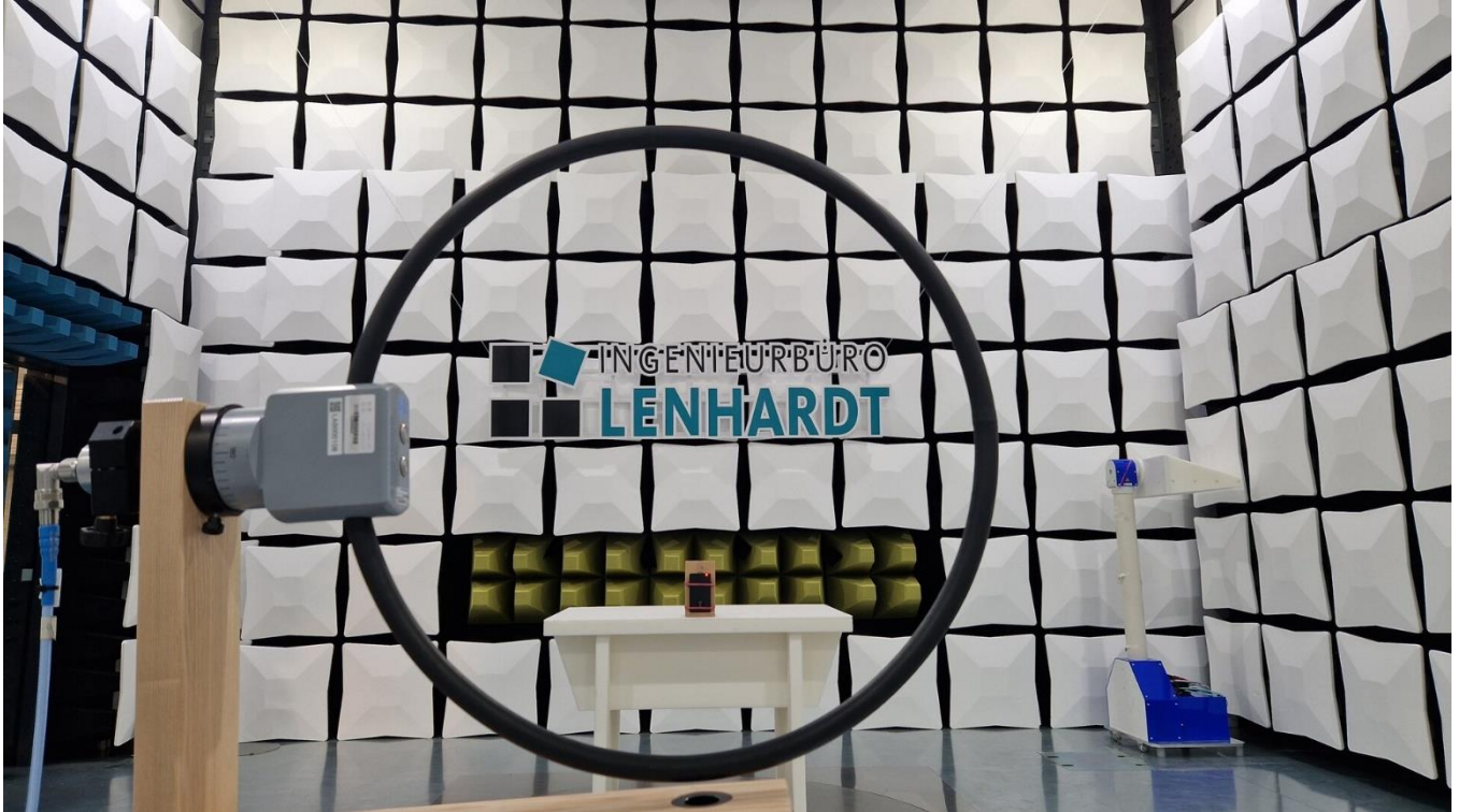
Photo No. 8, measurement in SAC, 9 kHz – 30 MHz, overall view:
