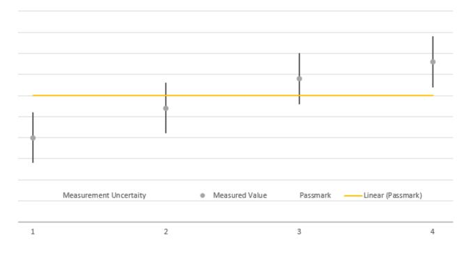
The verdicts in this test report are given according the above diagram:
