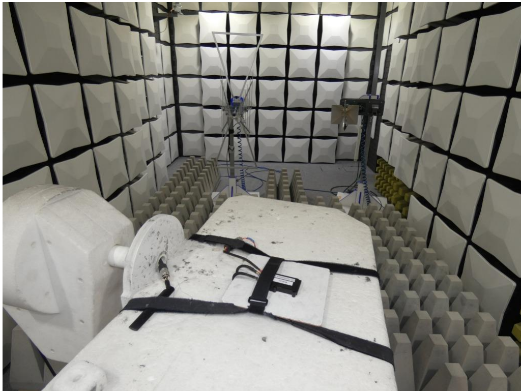
Photo 3: Test setup for radiated measurements above 1 GHz
