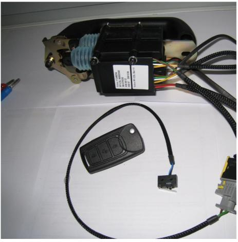
Picture 1 shows the door lock mechanism with tow fitted motors and CDL-OS controller with all connectors, the rotor switch, and the RF remote control transmitter key.
