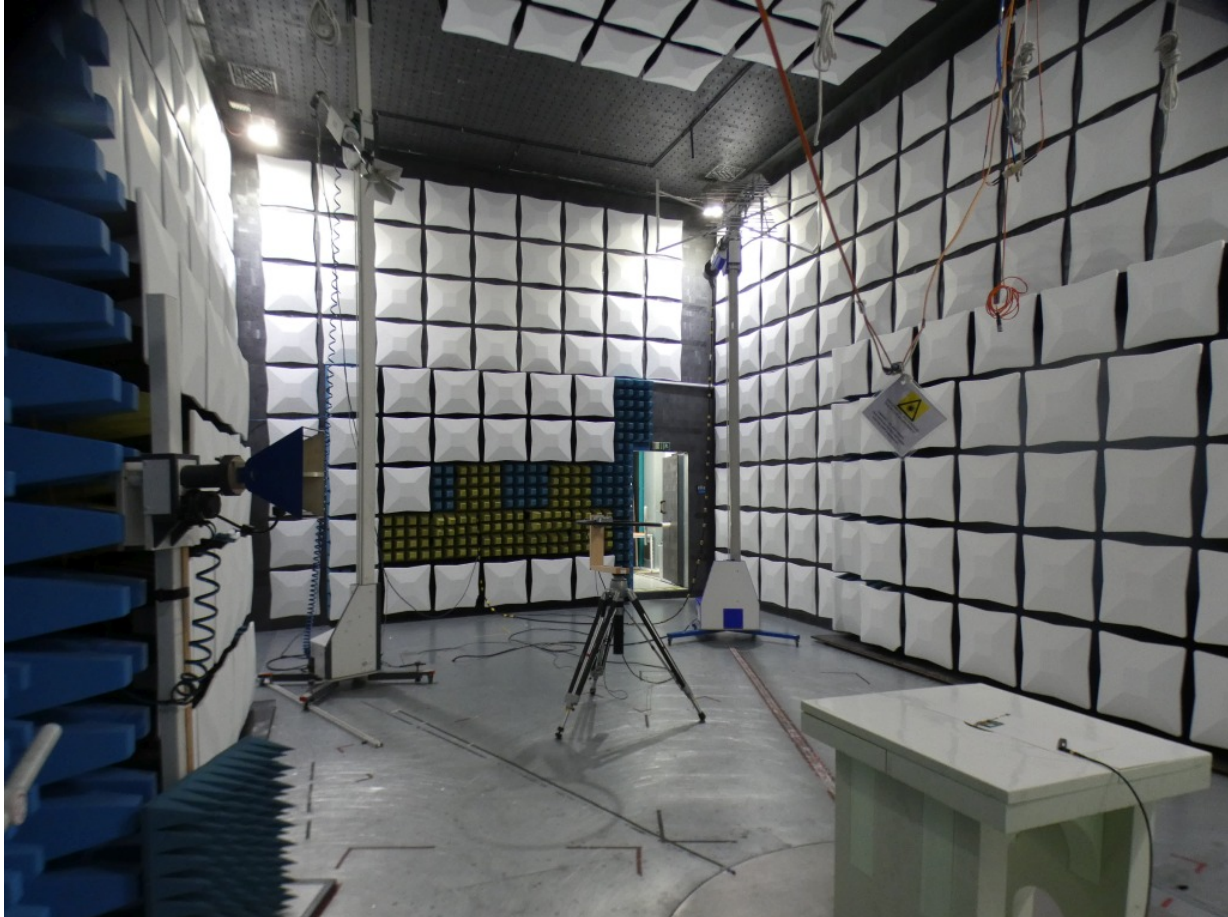
Photo 1: Test setup for radiated measurements (stand alone setup, 9 kHz - 30 MHz; FCC 15c247)
