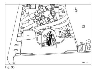
Switch on the main battery switch (Fig. 35).
