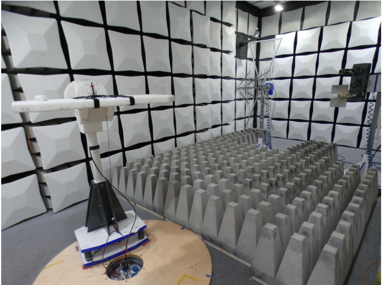
Photo 3: Test setup for radiated measurements (stand alone setup, 1 GHz – 24 GHz; FCC 15c247)
