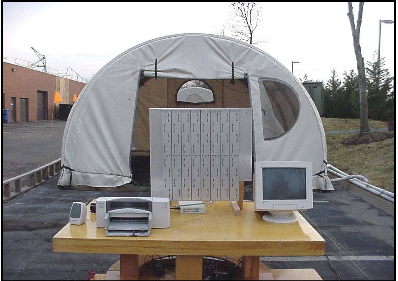
PHOTOGRAPH 3: RADIATED TEST FRONT VIEW
