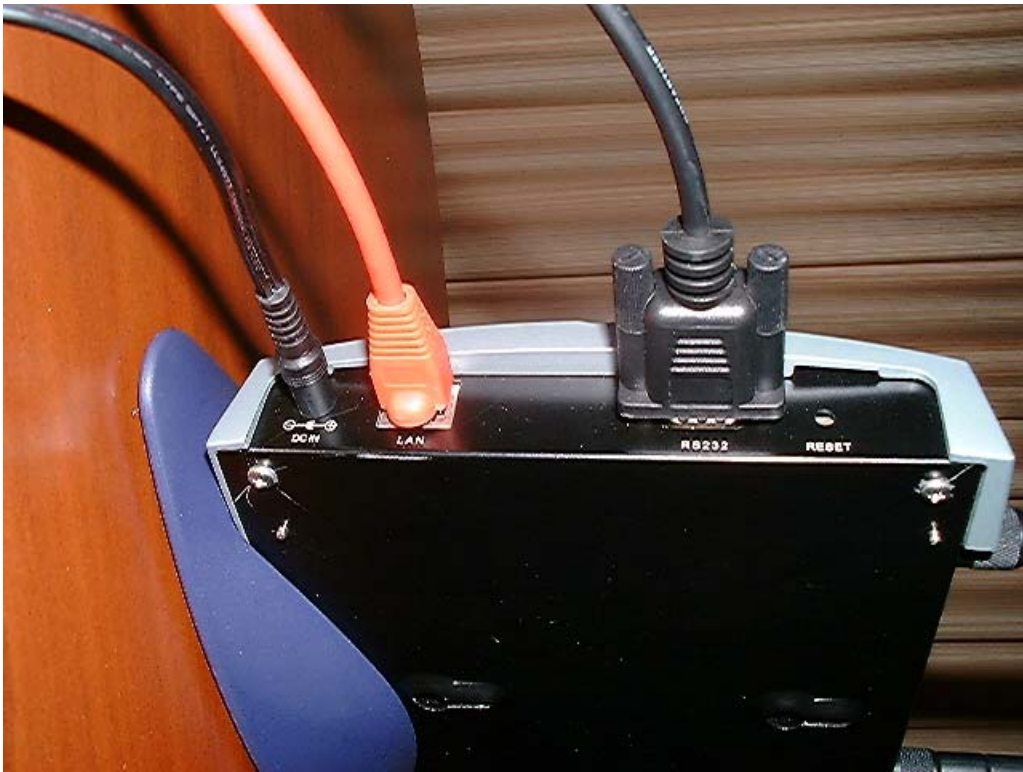
Figure 11 - I/O port s with cables attached
