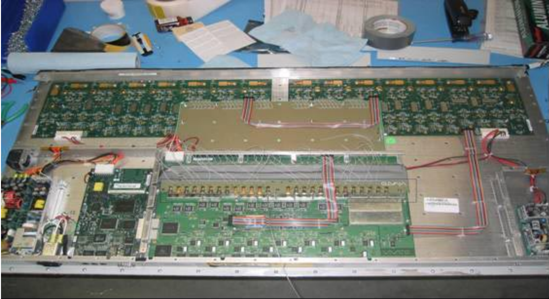
Figure4: Internal view of Vivato Wi-Fi Switch. The board in the black rectangle in the middle of the picture is the adapter board used to inject the signal for the measurement
