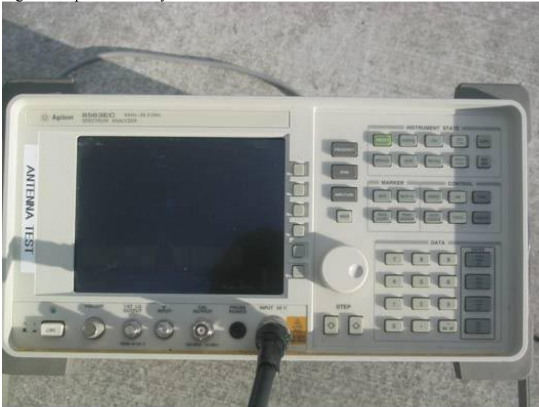
Figure 9: Spectrum analyzer used to make the measurement
