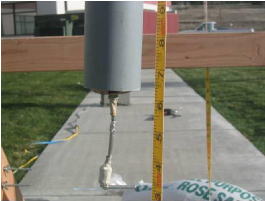
Figure 7 : Closeup of measurement dipole
