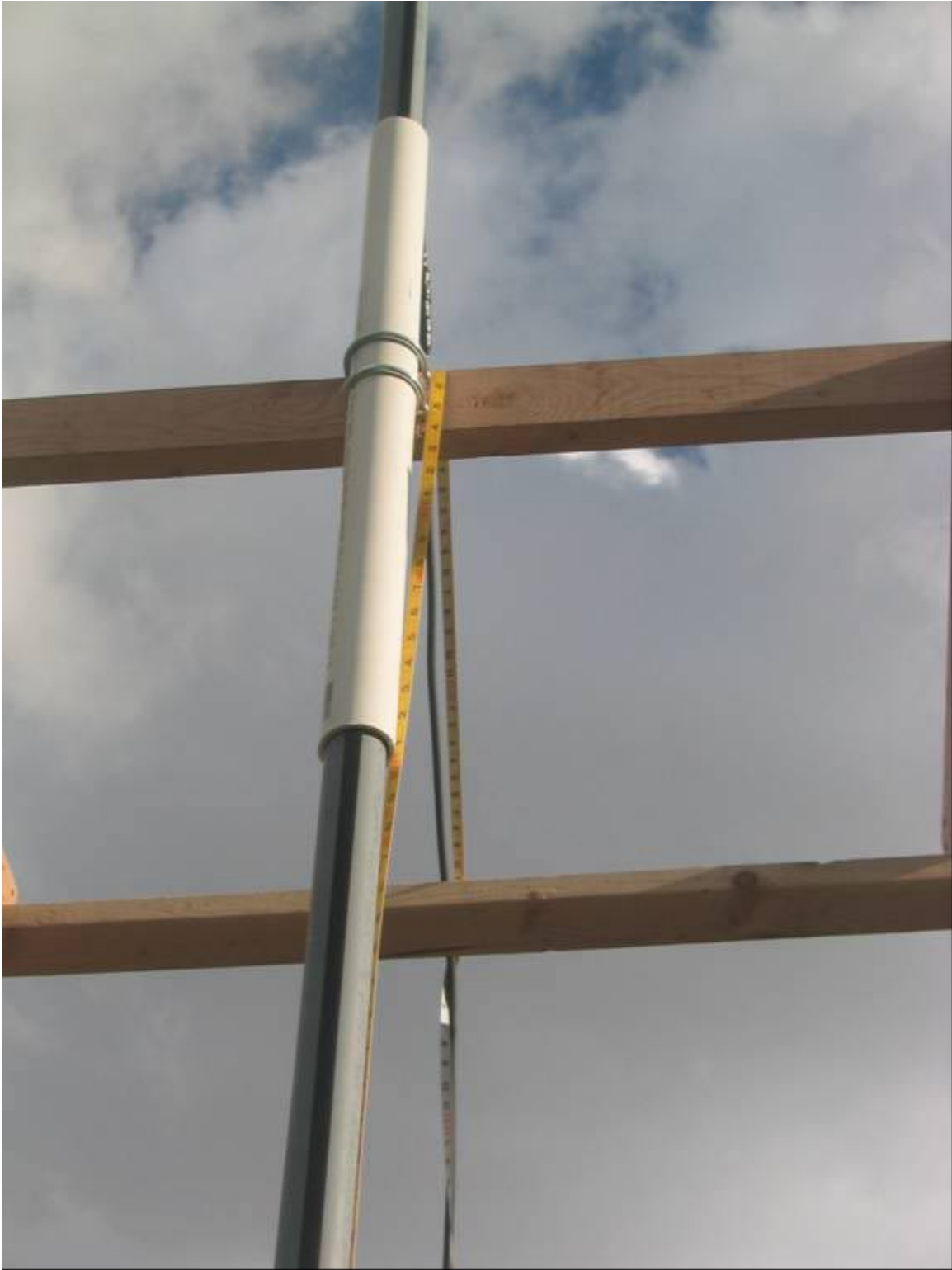
Figure 8: Sliding Linear bearing. Black strip is a made of Velcro and provides a friction fit holding the gray PVC pipe section in place
