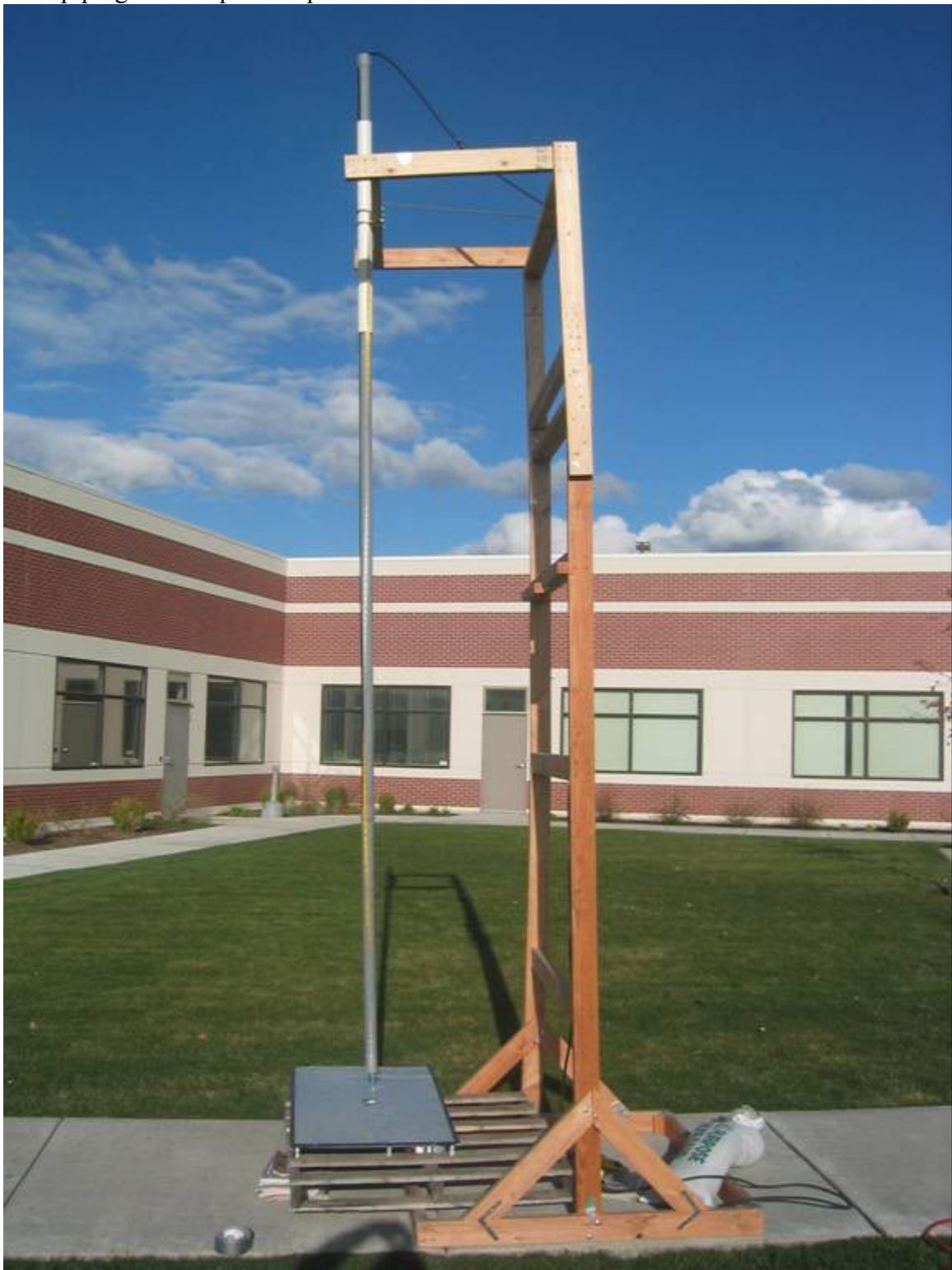
Figure2: Side view if the measurement apparatus. The linear bearing is the white piece of PVC piping at the top of the picture.
