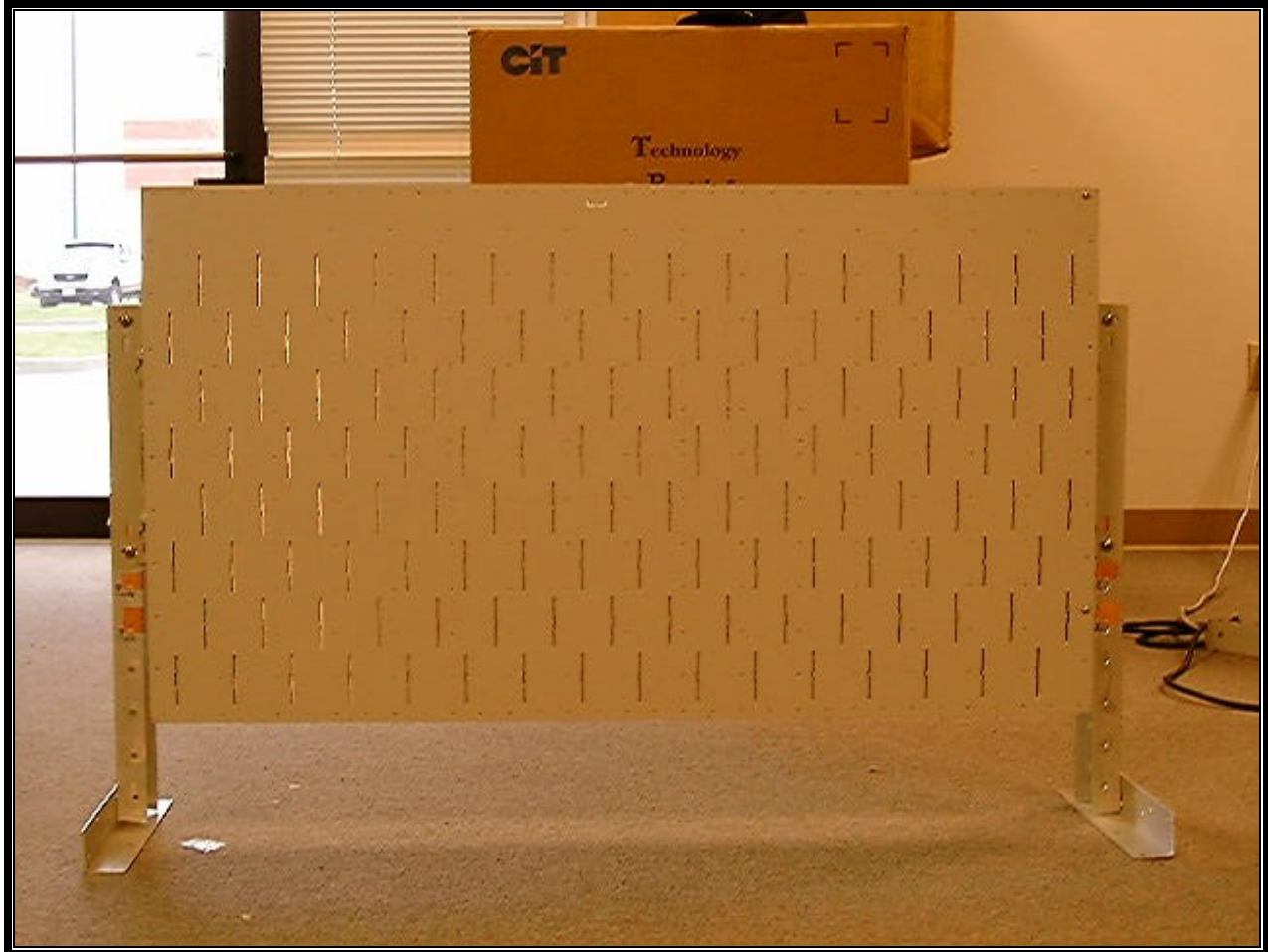
PHOTOGRAPH 5: FRONT OF WI-FI SWITCH SHOWING SLOT ANTENNAS
