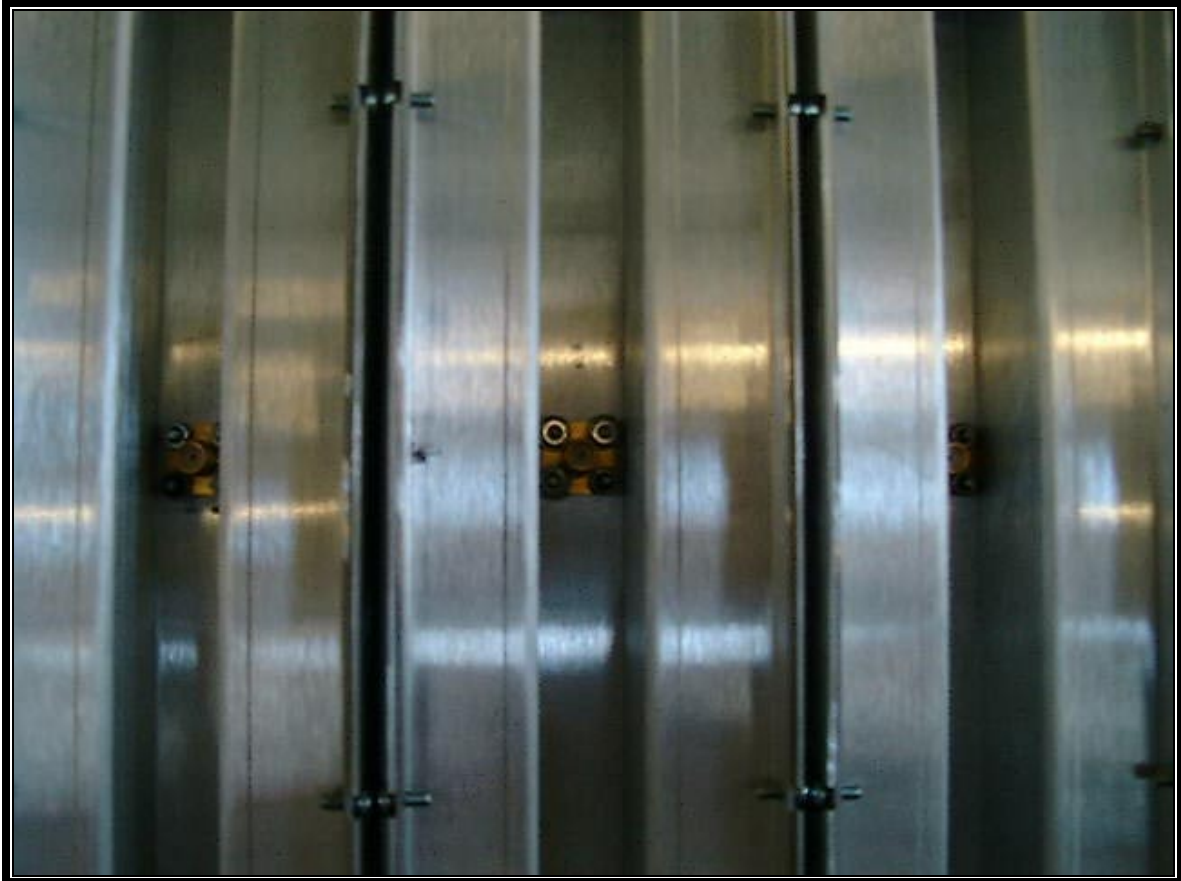
PHOTOGRAPH 53: SMA INPUT TO ANTENNA ELEMENT
