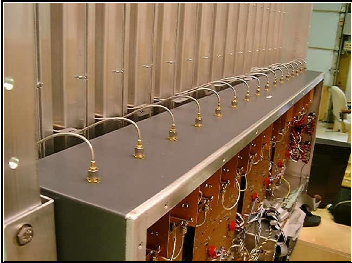
PHOTOGRAPH 54: RF PORT TO ANTENNA
