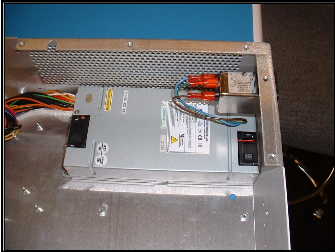
PHOTOGRAPH 15: AC LINE FILTER IMPLEMENTATION #1
