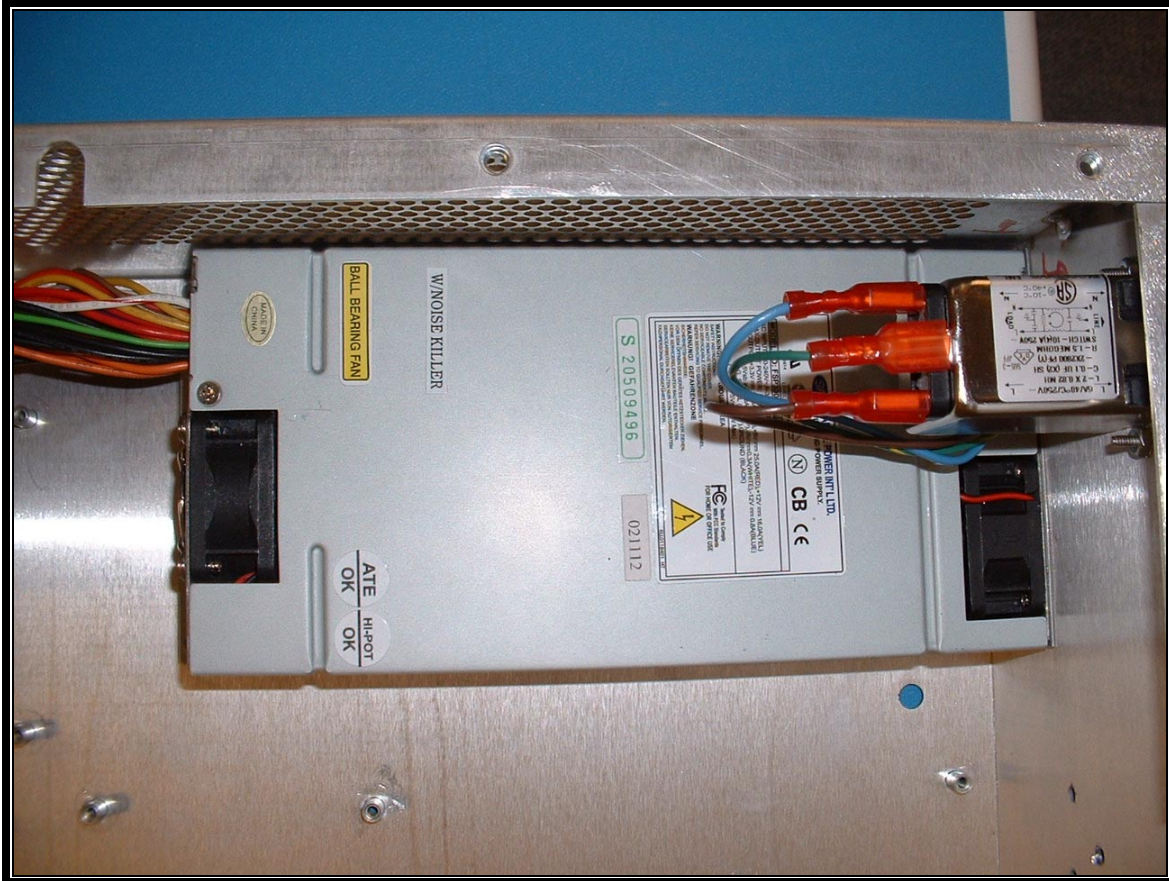
PHOTOGRAPH 18: AC LINE FILTER IMPLEMENTATION #4
