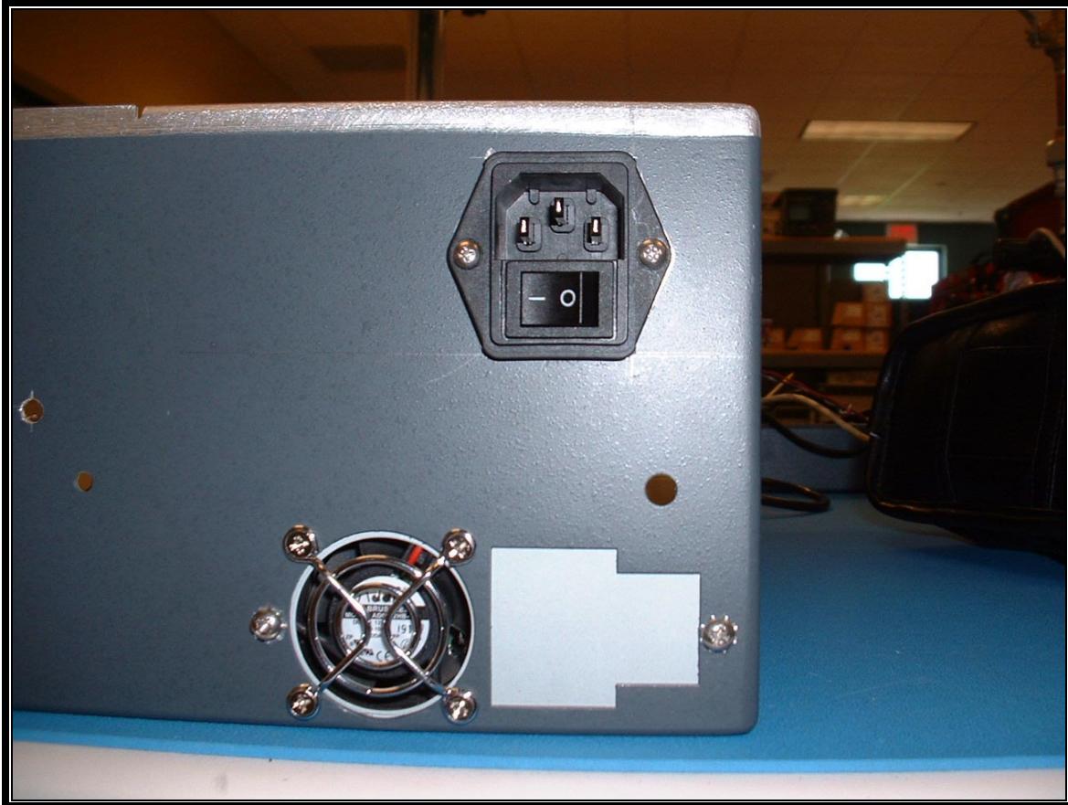
PHOTOGRAPH 17: AC LINE FILTER IMPLEMENTATION #3
