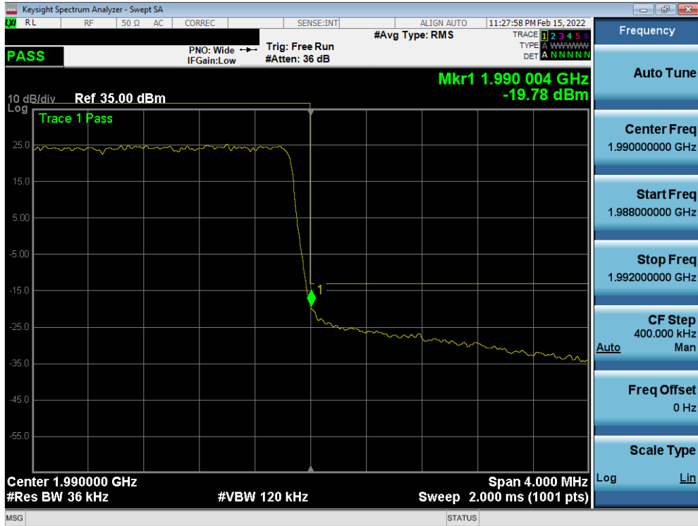
Plot 7-85. Upper Band Edge Plot (LTE Band 2 - 3MHz QPSK – Full RB - Ant1)
