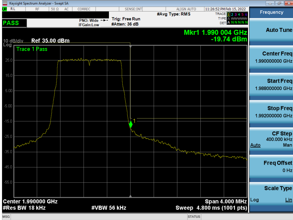
Plot 7-89. Upper Band Edge Plot (LTE Band 2 – 1.4MHz QPSK – Full RB - Ant1)
