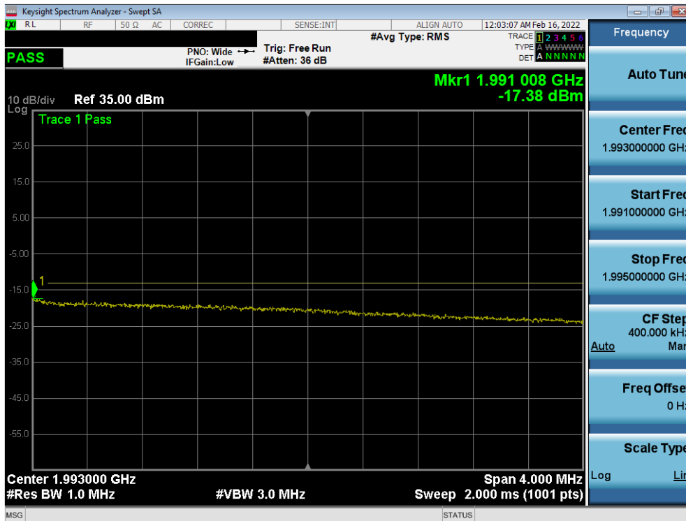
Plot 7-74. Extended Upper Band Edge Plot (LTE Band 2 - 15MHz QPSK – Full RB - Ant1)
