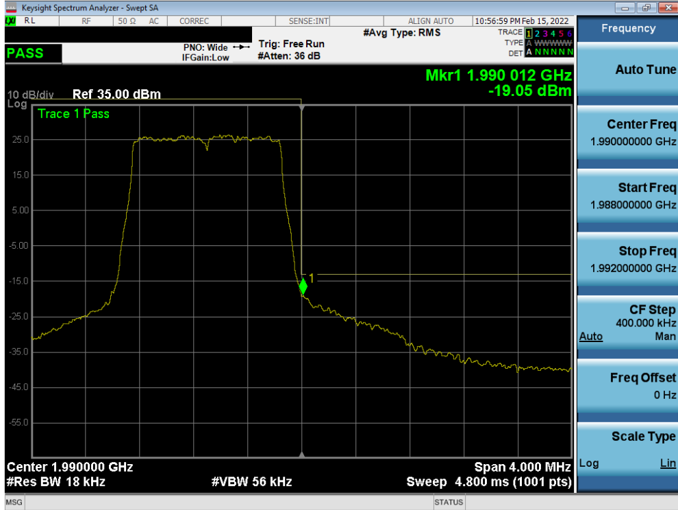
Plot 7-113. Upper Band Edge Plot (LTE Band 2 – 1.4MHz QPSK – Full RB - Ant2)
