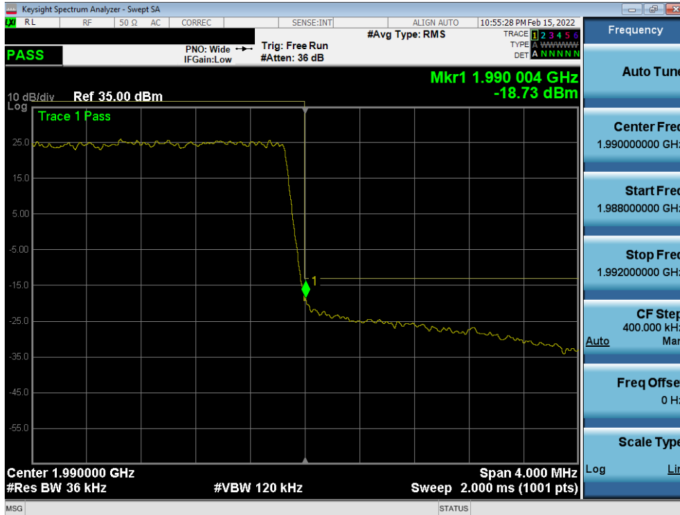
Plot 7-109. Upper Band Edge Plot (LTE Band 2 - 3MHz QPSK – Full RB - Ant2)
