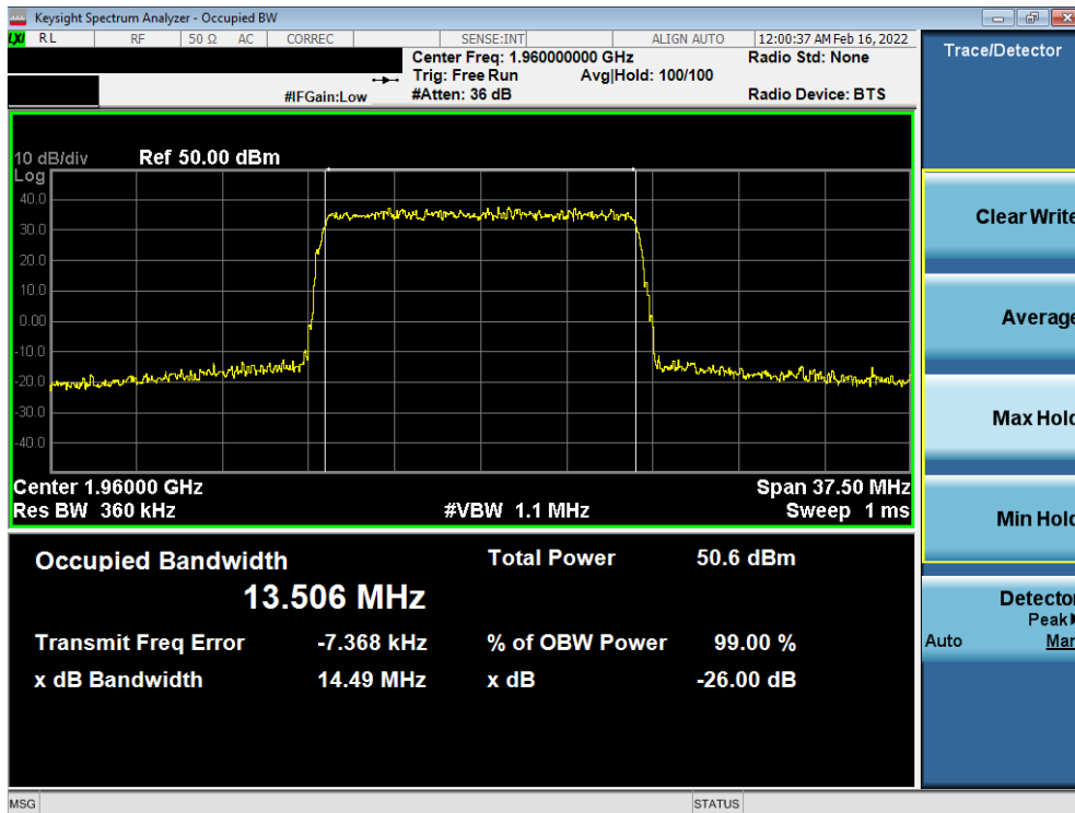
Plot 7-6. Occupied Bandwidth Plot (LTE Band 2 - 15MHz 16-QAM - Full RB - Ant1)
