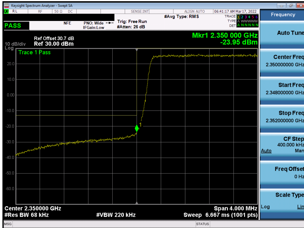
Plot 7-26. Lower Band Edge Plot (LTE Band 30 - 5MHz QPSK – Full RB Configuration)
