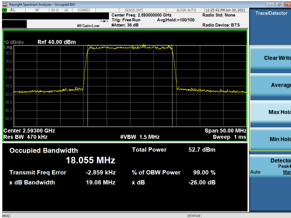
Plot 7-12. Occupied Bandwidth Plot (LTE Band 41 - 20MHz 16-QAM - Full RB)
