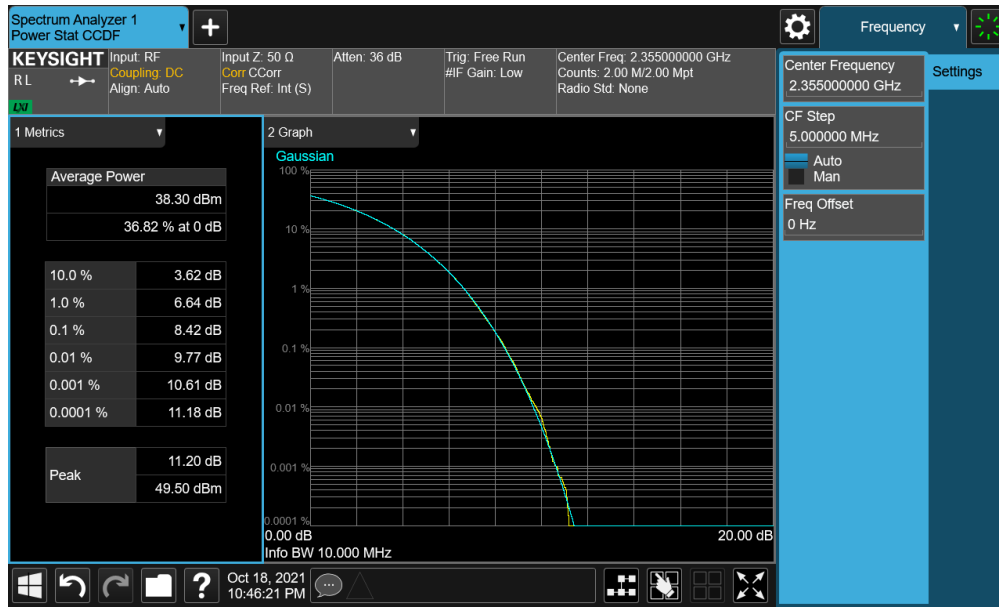
Plot 7-59. PAR Plot (Band 30 - 10.0MHz QPSK - Full RB Configuration)
