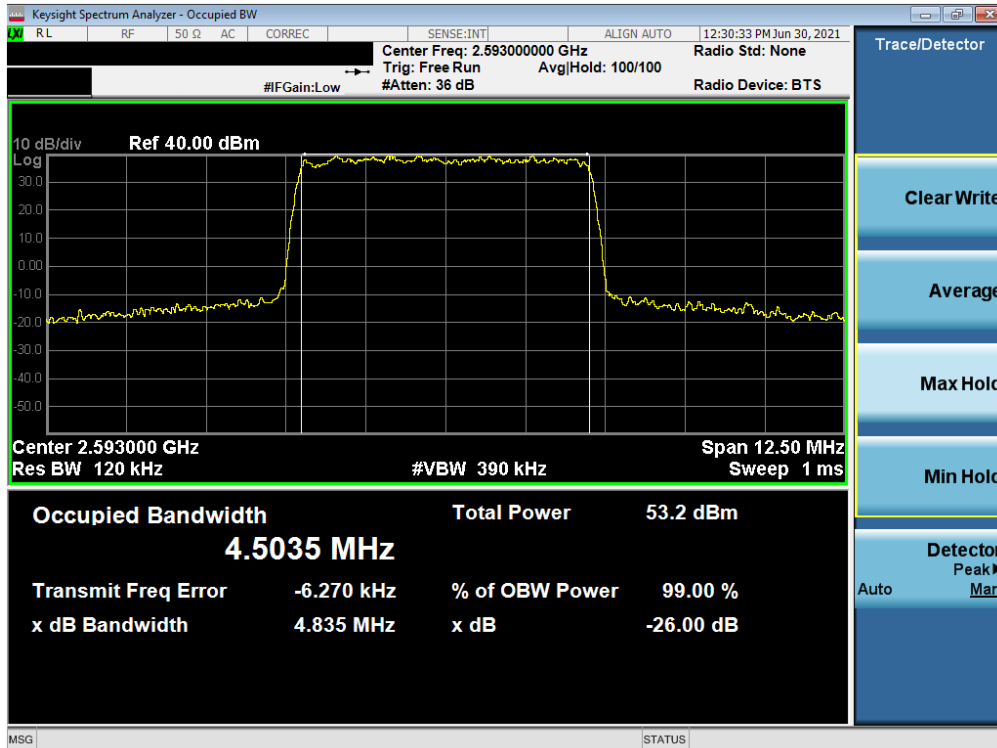
Plot 7-18. Occupied Bandwidth Plot (LTE Band 41 - 5MHz 16-QAM - Full RB)
