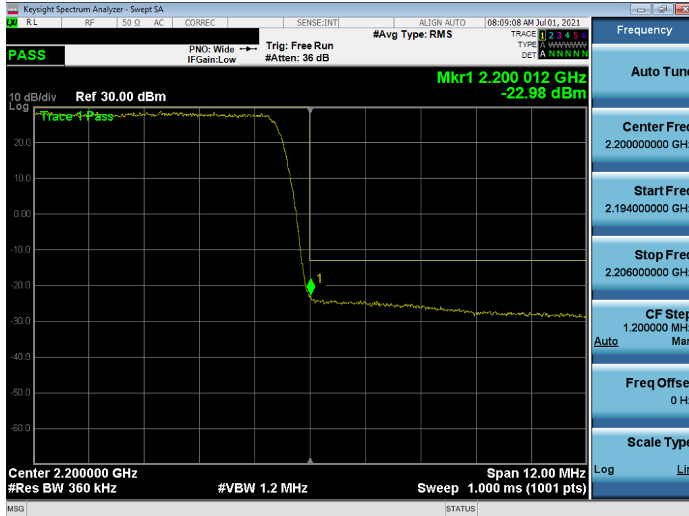
Plot 7-36. Upper Band Edge Plot (LTE Band 66 - 15MHz QPSK – Full RB)
