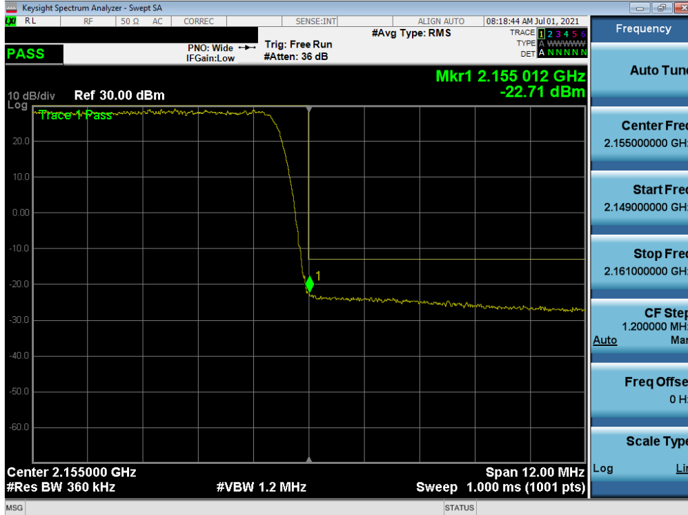
Plot 7-32. Upper Band Edge Plot (LTE Band 4 - 15MHz QPSK – Full RB)
