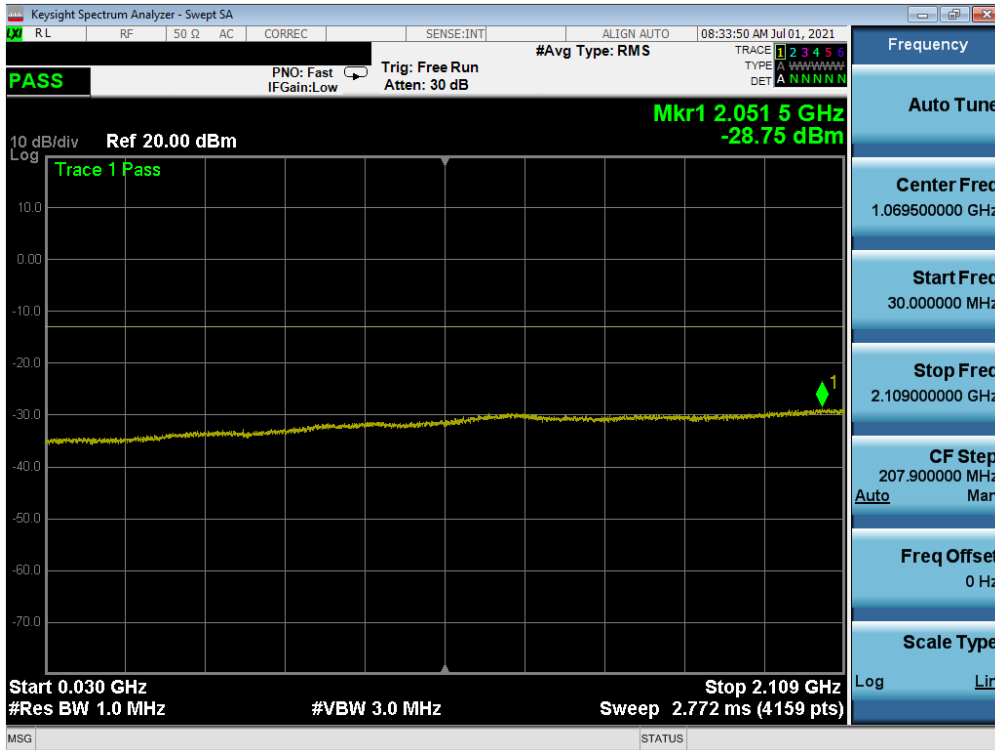
Plot 7-13. Conducted Spurious Plot (LTE Band 66/10/4 - 20MHz QPSK - 1 RB - Low Channel)
