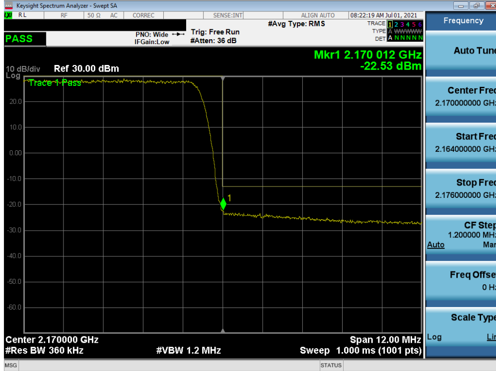
Plot 7-34. Upper Band Edge Plot (LTE Band 10 - 15MHz QPSK – Full RB)
