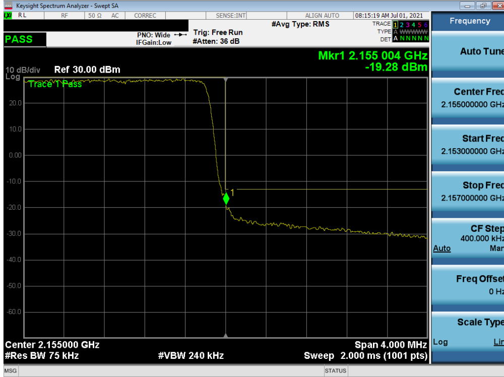
Plot 7-56. Upper Band Edge Plot (LTE Band 4 - 3MHz QPSK – Full RB)
