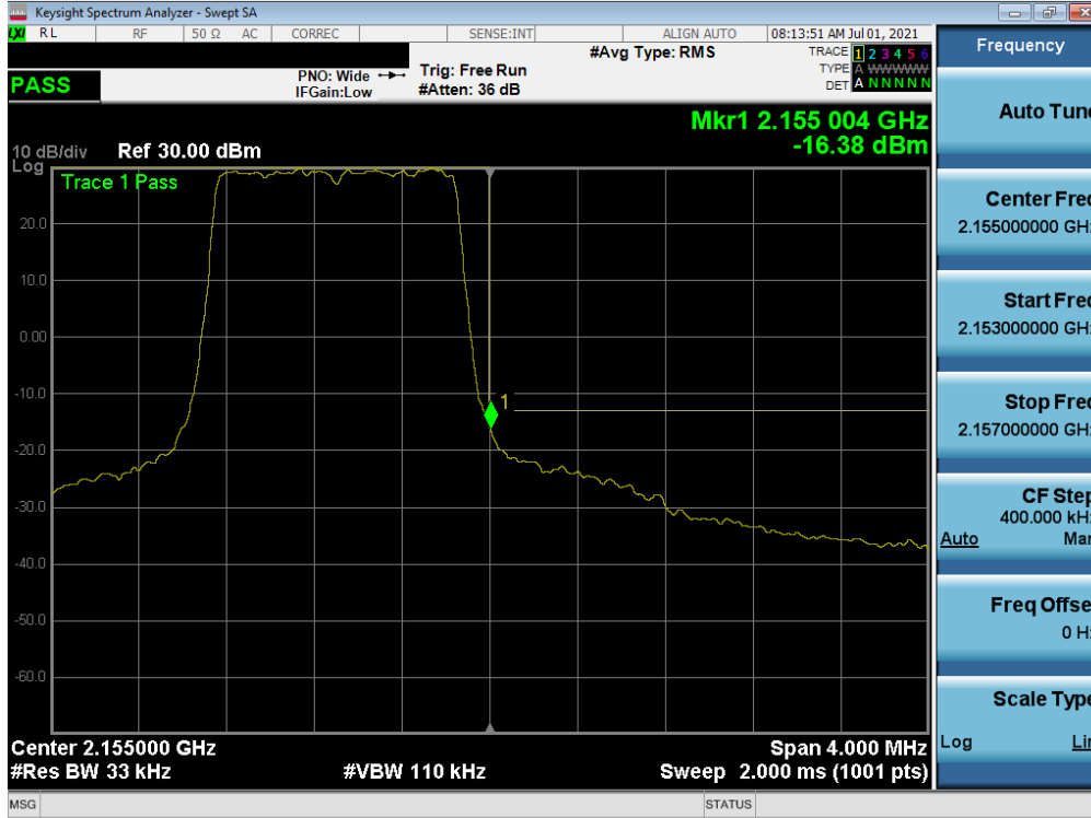
Plot 7-62. Upper Band Edge Plot (LTE Band 4 – 1.4MHz QPSK – Full RB)
