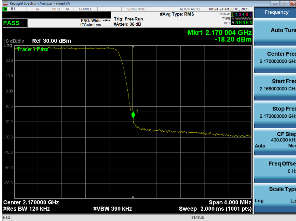
Plot 7-48. Upper Band Edge Plot (LTE Band 10 - 5MHz QPSK – Full RB)
