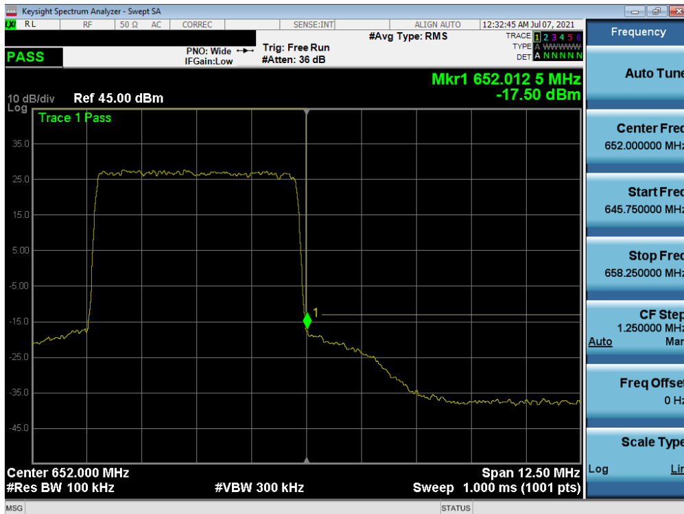
Plot 7-49. Upper Band Edge Plot (LTE Band 71 - 5MHz QPSK – Full RB)
