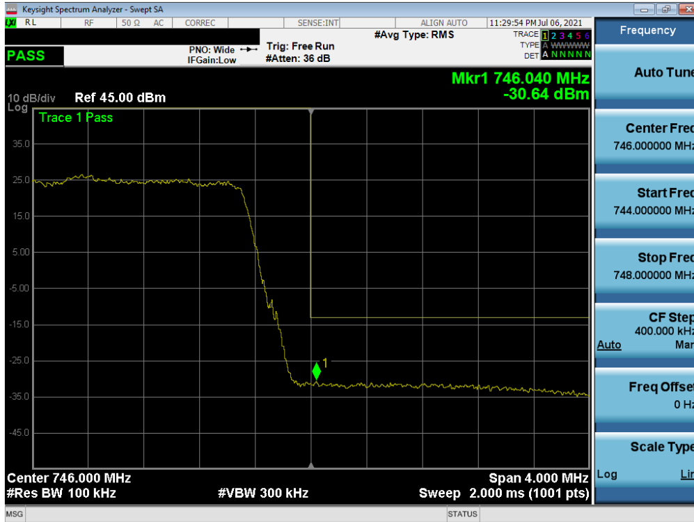
Plot 7-52. Upper Band Edge Plot (LTE Band 12/17 - 10MHz QPSK – Full RB)
