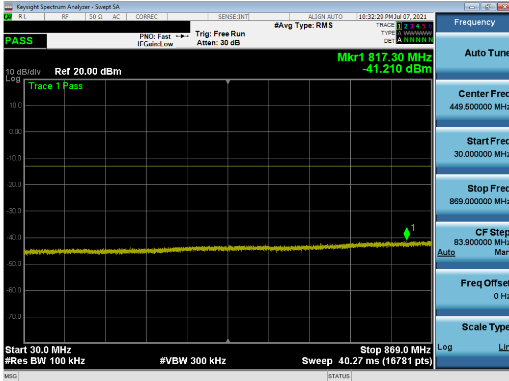
Plot 7-17. Conducted Spurious Plot (LTE Band 26/5 - 10MHz QPSK - Full RB - High Channel)
