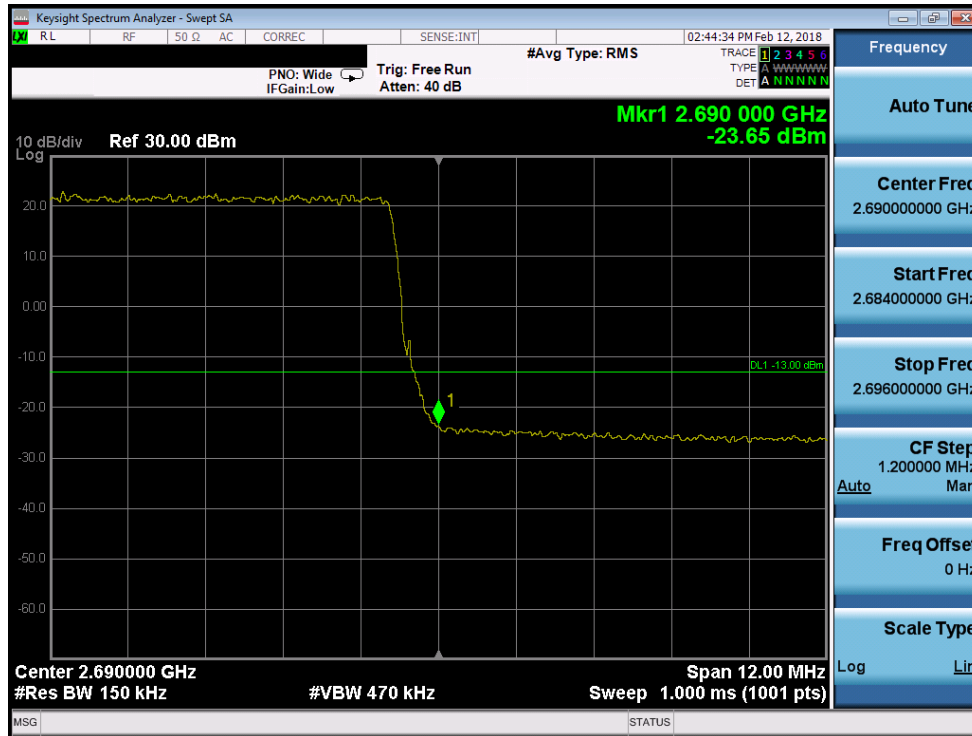
Plot 7-253. Upper Band Edge Plot (Band 41 - 15.0MHz 64-QAM)
