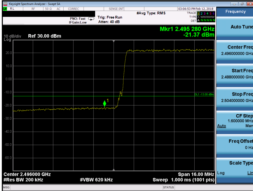
Plot 7-259. Lower Band Edge Plot (Band 41 - 20.0MHz QPSK)
