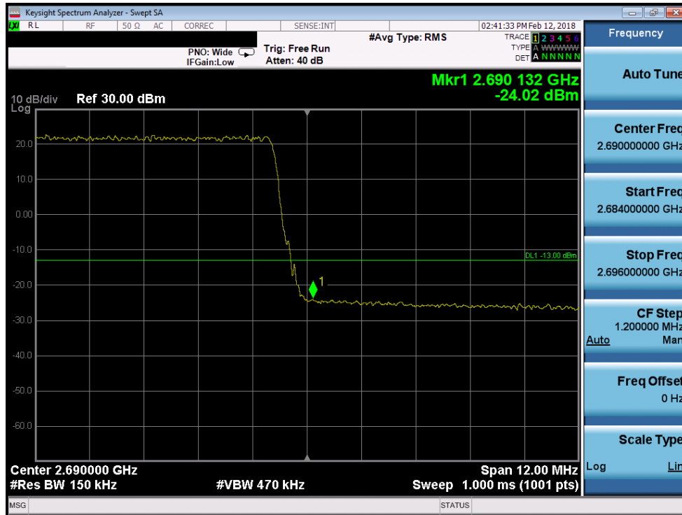
Plot 7-245. Upper Band Edge Plot (Band 41 - 15.0MHz QPSK)
