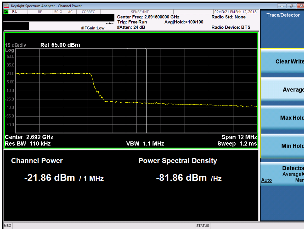
Plot 7-250. Upper Extended Band Edge Plot (Band 41 - 15.0MHz 16-QAM)
