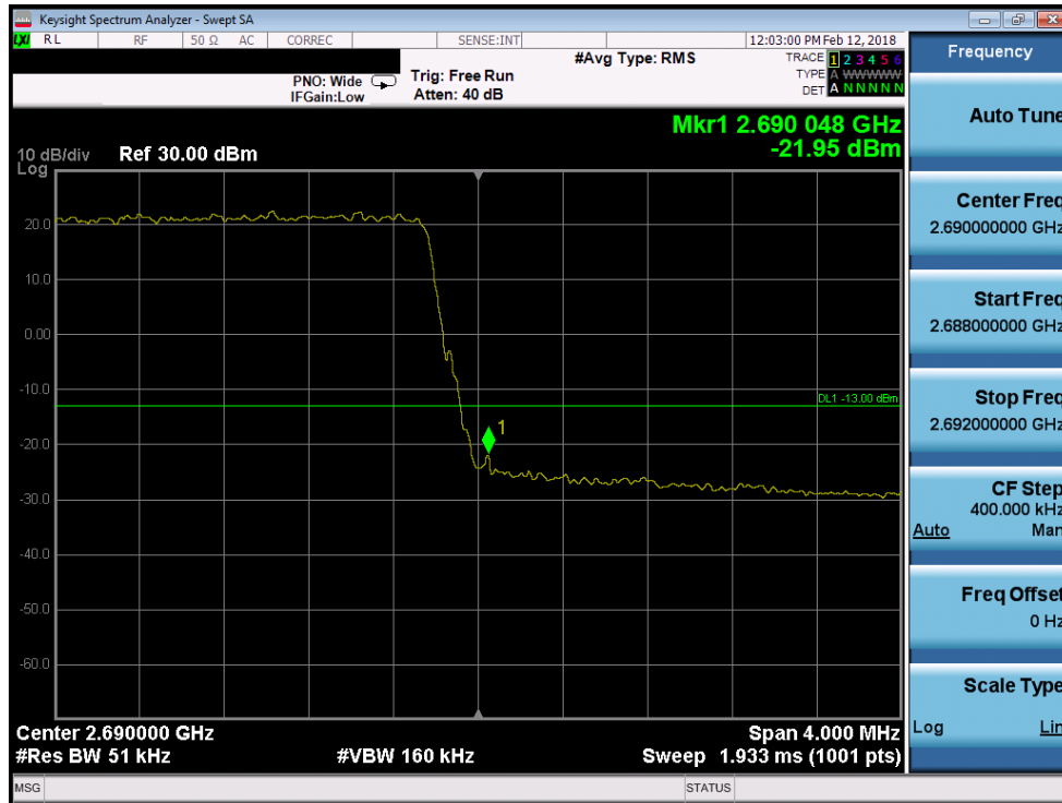
Plot 7-225. Upper Band Edge Plot (Band 41 - 5.0MHz 256-QAM)
