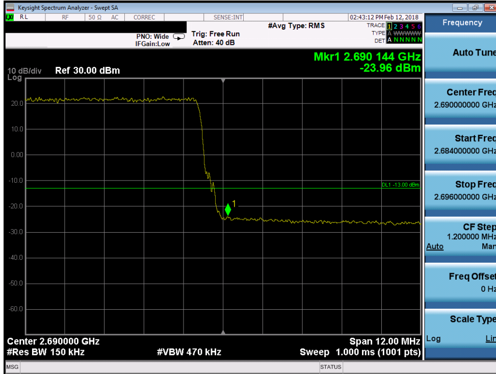
Plot 7-249. Upper Band Edge Plot (Band 41 - 15.0MHz 16-QAM)
