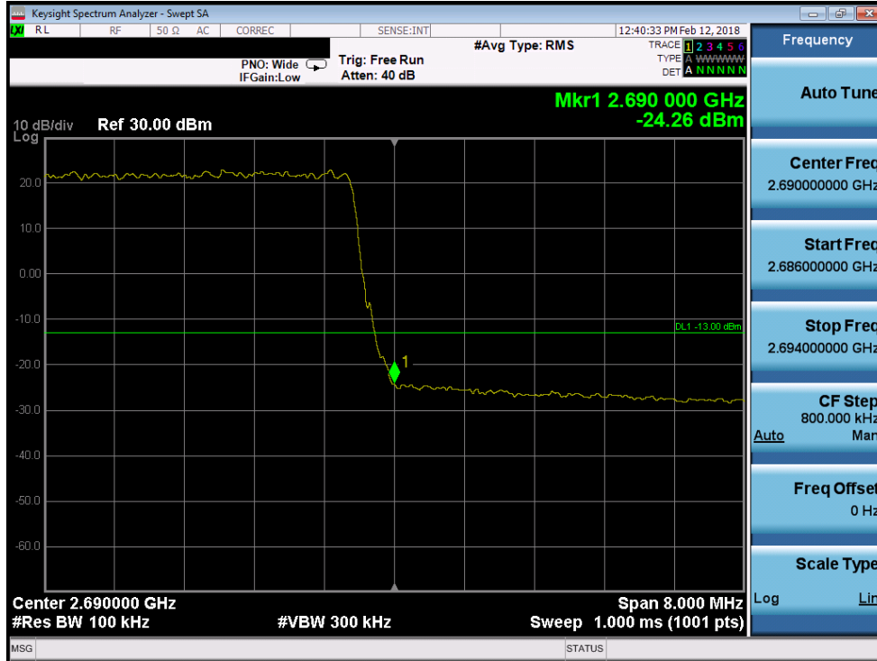
Plot 7-237. Upper Band Edge Plot (Band 41 - 10.0MHz 64-QAM)
