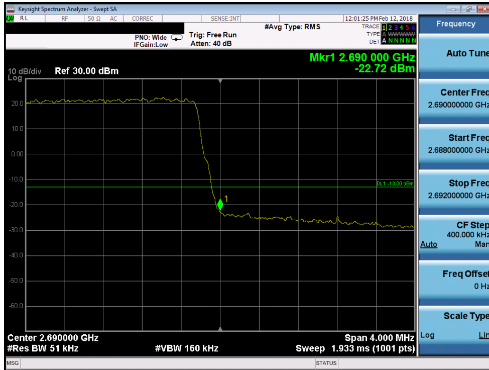
Plot 7-221. Upper Band Edge Plot (Band 41 - 5.0MHz 64-QAM)
