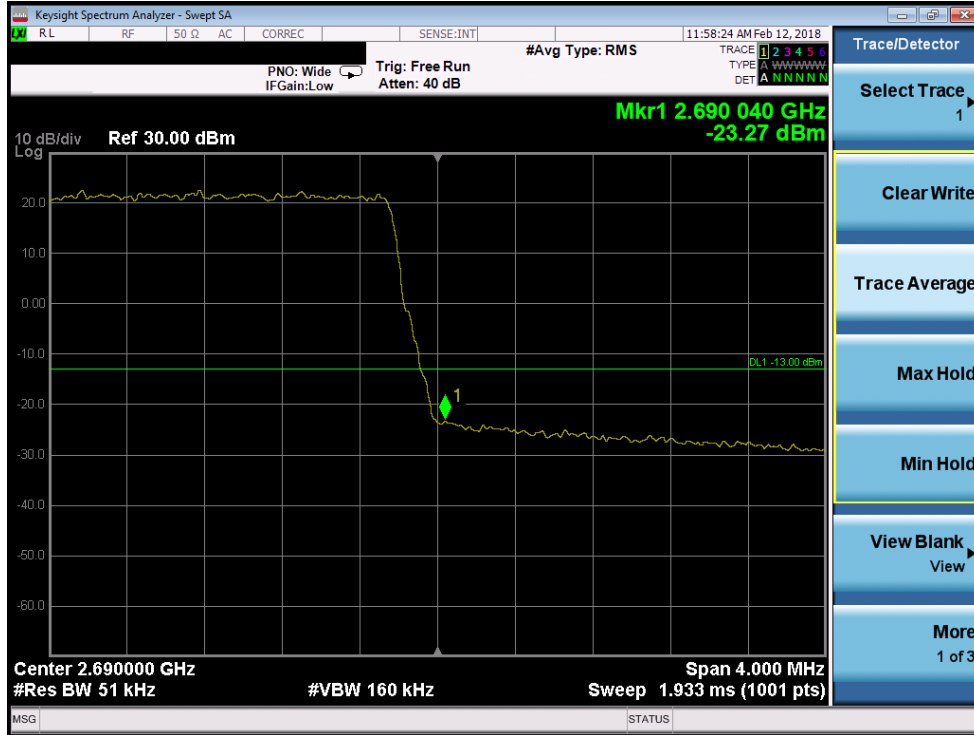
Plot 7-213. Upper Band Edge Plot (Band 41 - 5.0MHz QPSK)
