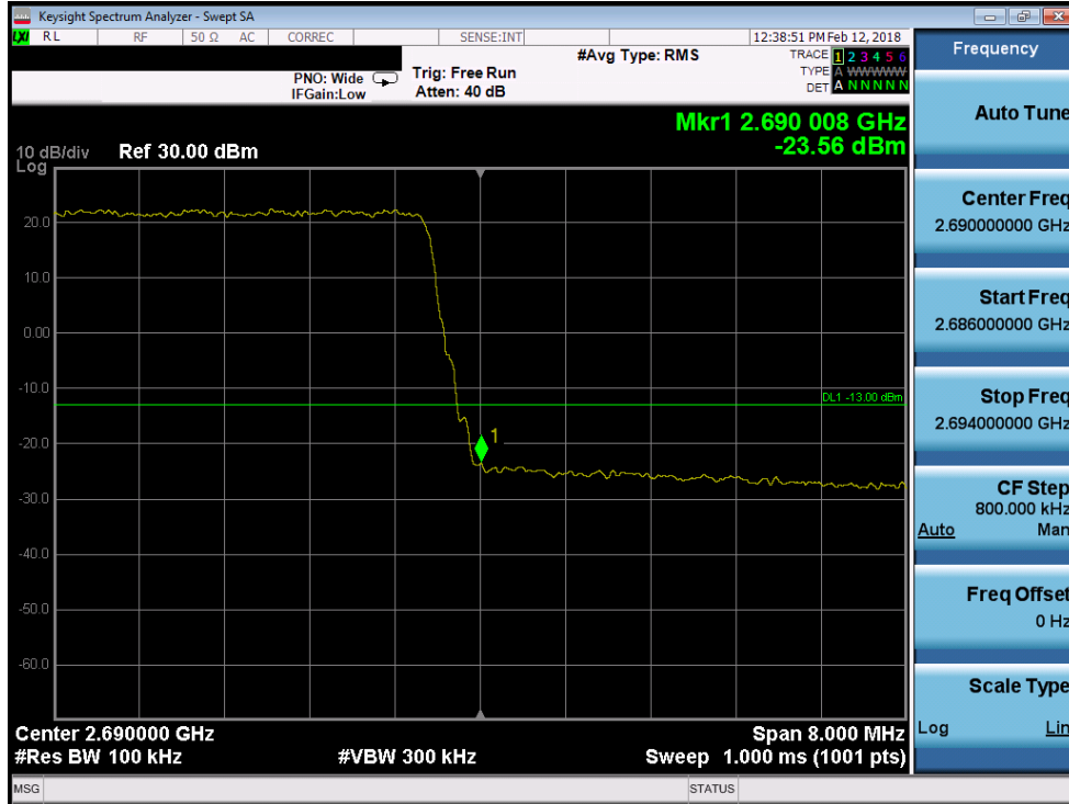
Plot 7-233. Upper Band Edge Plot (Band 41 - 10.0MHz 16-QAM)
