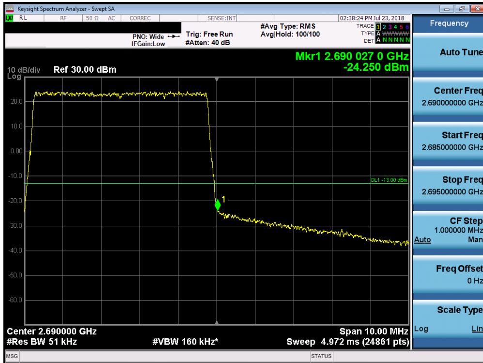
Plot 7-153. Upper Band Edge Plot (Band 7 - 5.0MHz 16-QAM)
