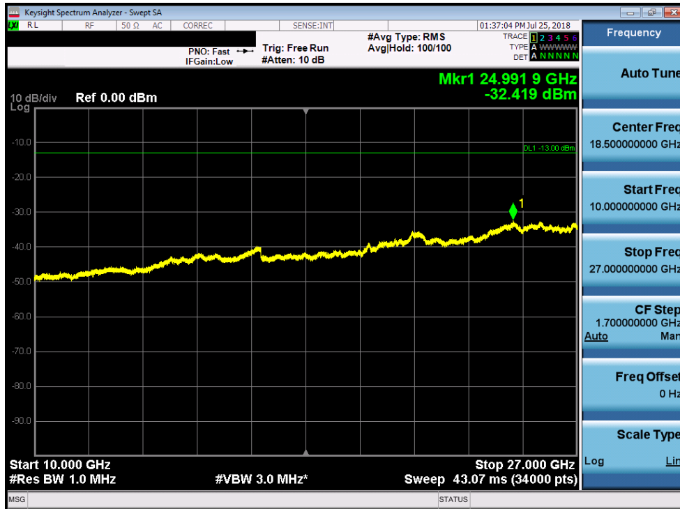
Plot 7-131. Conducted Spurious Plot (Band 7 - 10.0MHz QPSK – Low Channel)
