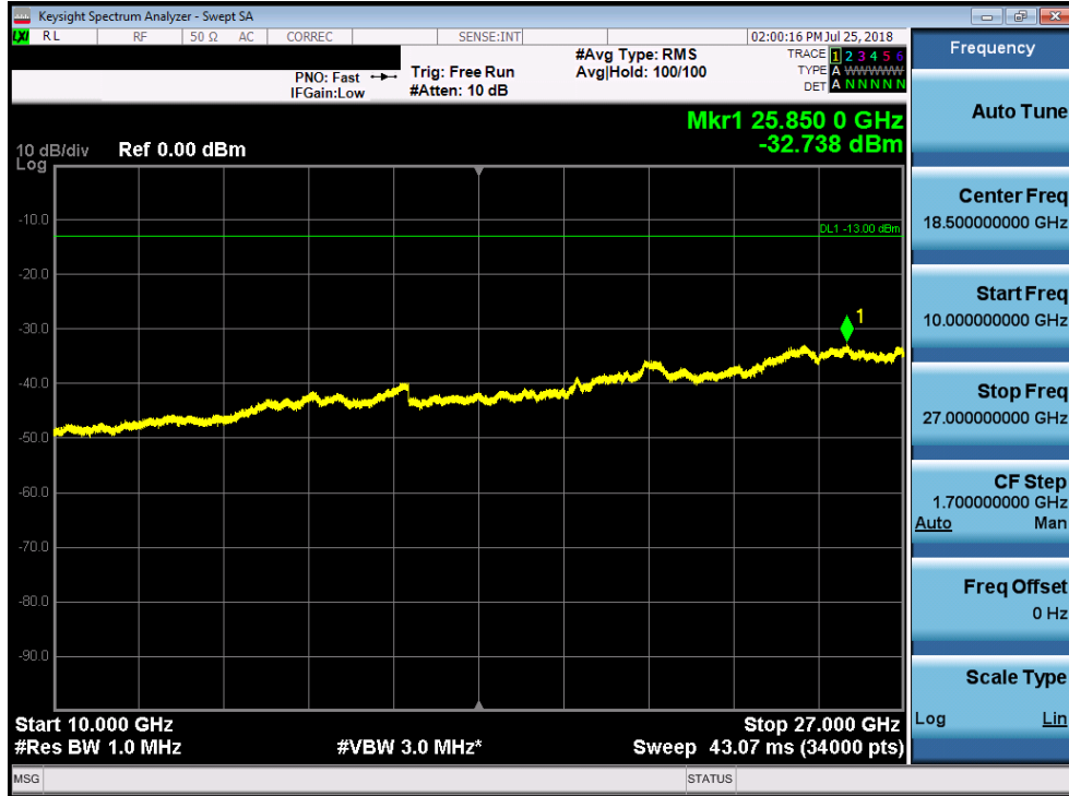
Plot 7-140. Conducted Spurious Plot (Band 7 - 10.0MHz QPSK – Low Channel)
