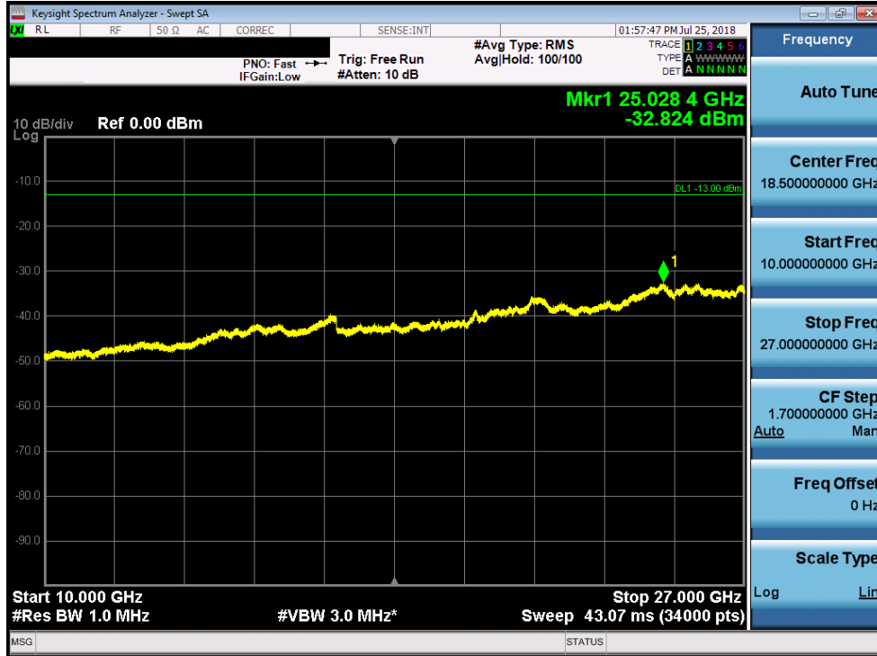
Plot 7-146. Conducted Spurious Plot (Band 7 - 10.0MHz QPSK – High Channel)
