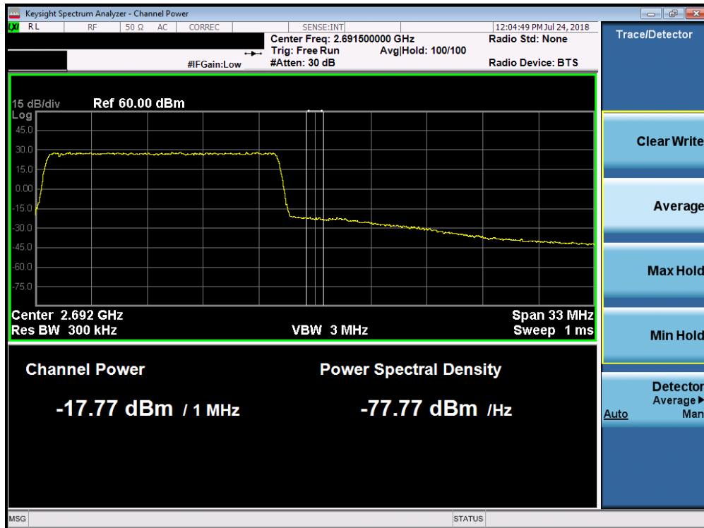
Plot 7-182. Upper Extended Band Edge Plot (Band 7 - 15.0MHz QPSK)
