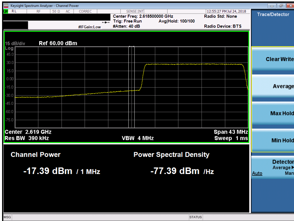
Plot 7-196. Lower Extended Band Edge Plot (Band 7 - 20.0MHz QPSK)
