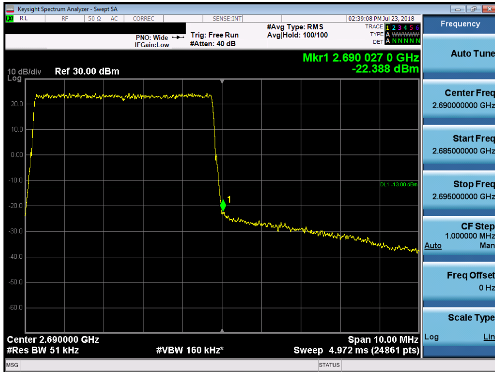
Plot 7-161. Upper Band Edge Plot (Band 7 - 5.0MHz 256-QAM)
