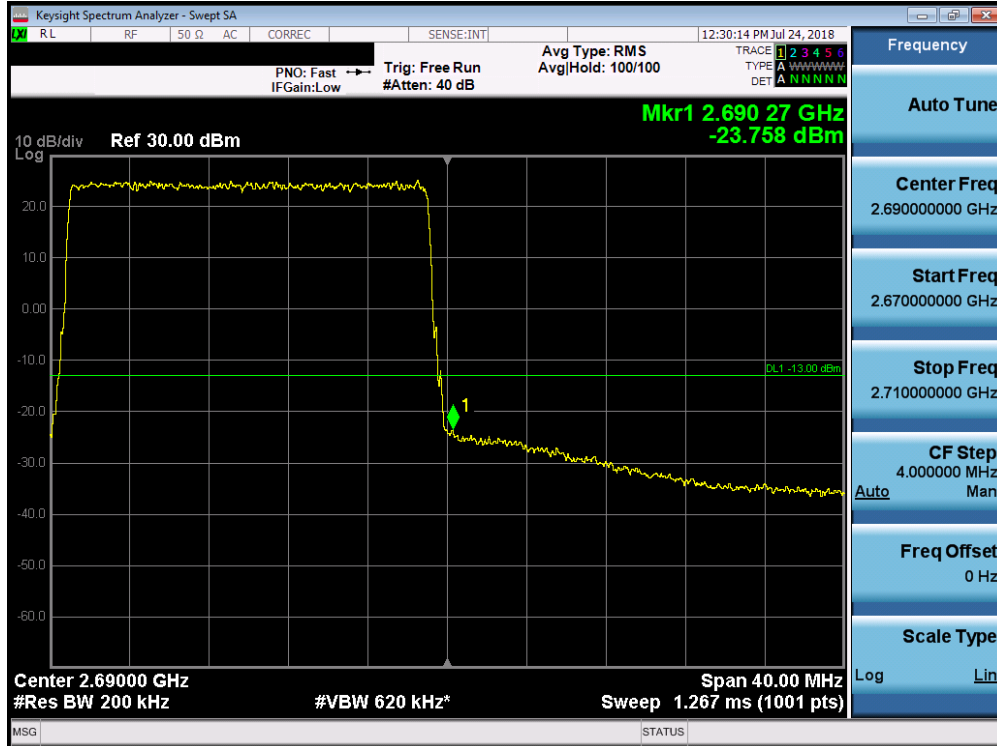
Plot 7-201. Upper Band Edge Plot (Band 7 - 20.0MHz 16-QAM)
