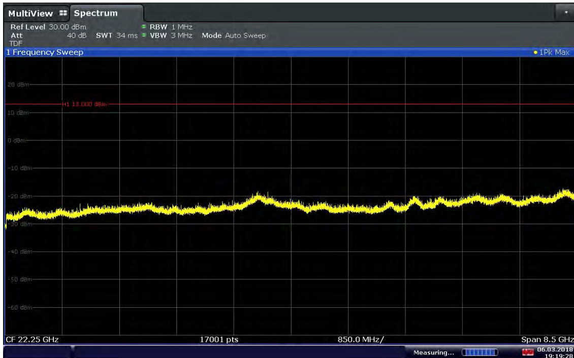
Plot 7-454. Radiated Spurious Plot above 18GHz (Band 2 – Mid Channel - 5.0MHz QPSK, Ant. Pol. V)
