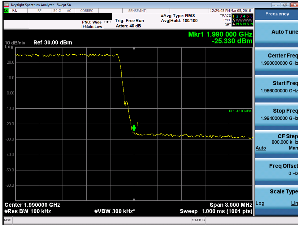
Plot 7-365. Upper Band Edge Plot (Band 2 - 10.0MHz 64-QAM)
