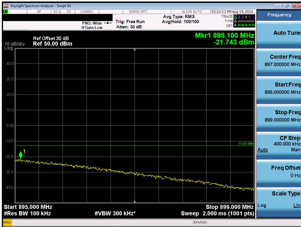
Plot 7-16. 4MHz Span Plot (Cellular UMTS Mode – Ch. 4458)
