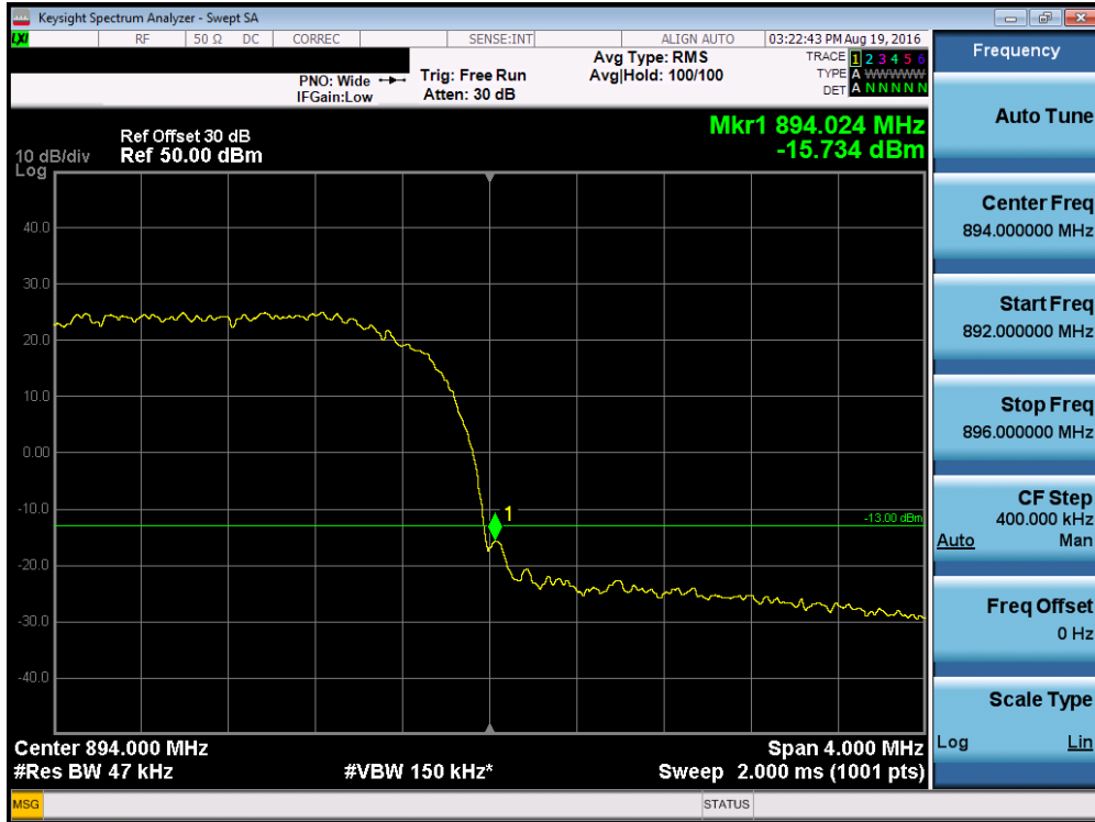
Plot 7-15. Band Edge Plot (Cellular UMTS Mode – Ch. 4458)
