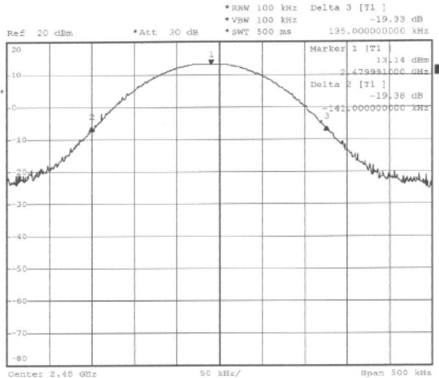
Observation : All emissions in any 100kHz bandwidth outside the band edge are attenuated more then 20dB from the carrier.
