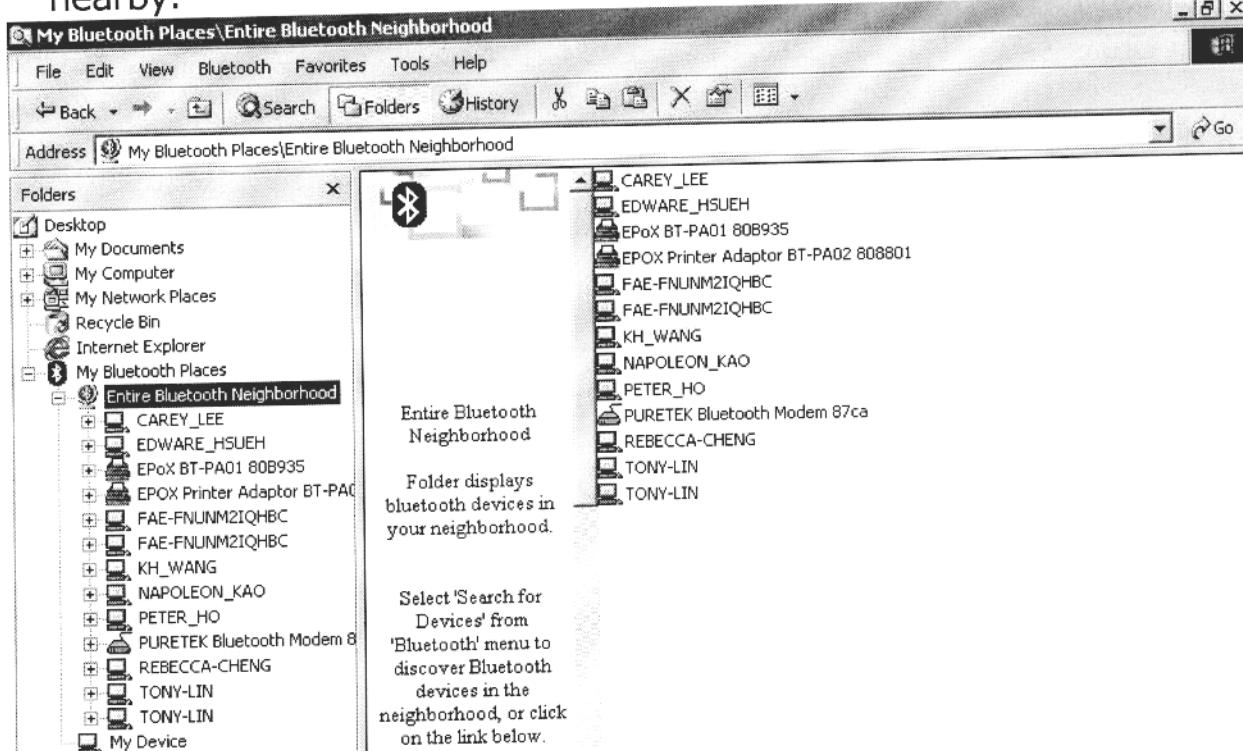
3 Find the **EPoX BT-PA01 XXXXXX** and double-click on it, the **Cable Replacement** icon be shown along with all the services offered by the printer adapter.
