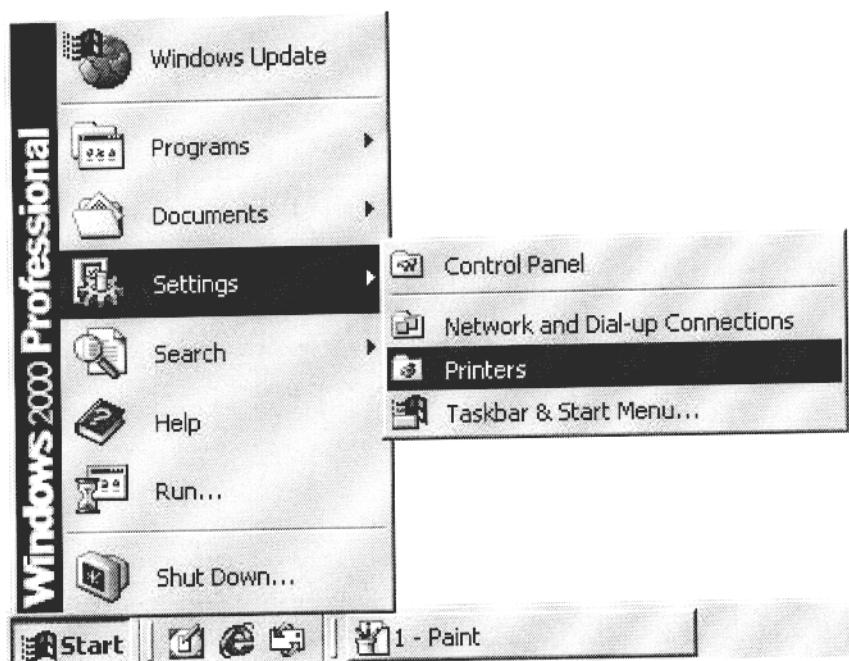
2. Please select the printer connected to the BT-PA01, and right-click on its icon, and then select **Properties** to enter the properties window.
