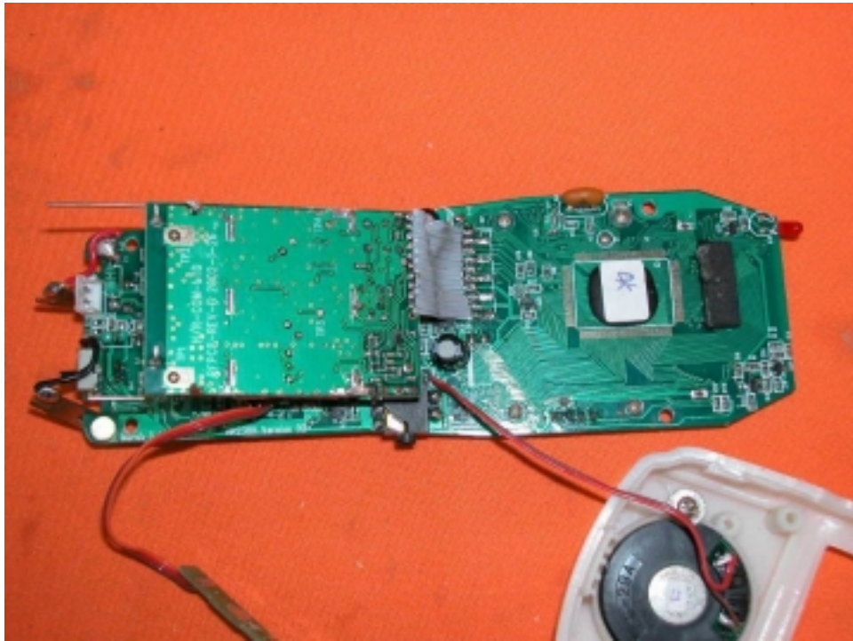
Handset Main PCB comp side (View 2)
