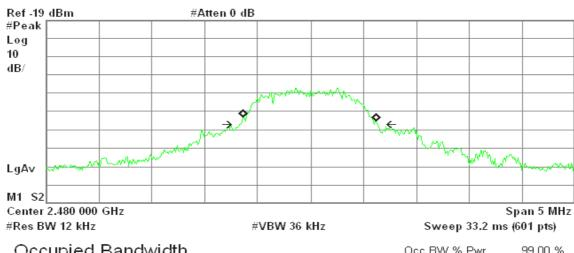
Occupied Bandwidth 1.2467 MHz Occ BW % Pwr 99.00 % x dB -20.00 dB
