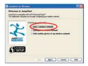
**Note:** There are two ways to setup WPS. One is by pushing the integrated WPS button on your router and the other is by entering the access PIN from your USB adapter to establish the WPS encryption with your router.
