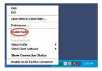
2. You may re-establish the Wi-Fi connection at anytime by selecting **Enable Radio**
