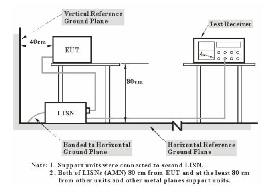
The setup of EUT is according with per ANSI C63.4-2003 measurement procedure. The specification used was with the FCC Part 15.207 limits.
