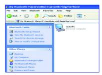
Double click on the device to display a list of its services. To establish a network connection, right click on Network Access and select Connect to Network Access Point.
