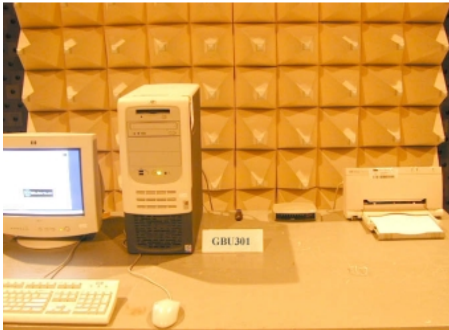
Photo 1: Spurious Test Set-up (front)
