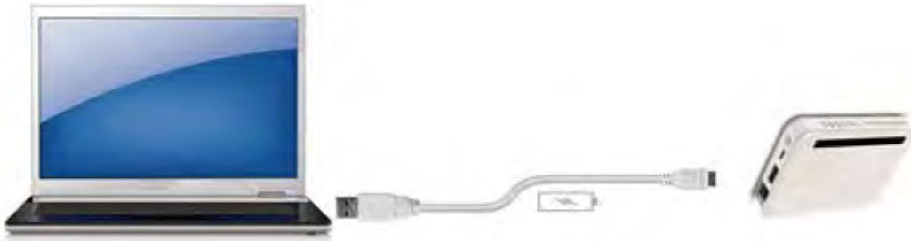
The Wi-Fi SD/USB works as SD memory card reader and charges the internal battery
