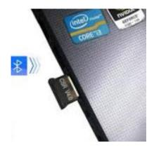
2. Windows 8 or 10 will automatically install the GBU522 device driver when the USB Bluetooth Adapter is installed. It will take a few moments to install the driver for the first time. You can check to see if the Bluetooth adapter has been successfully installed in device manager.
