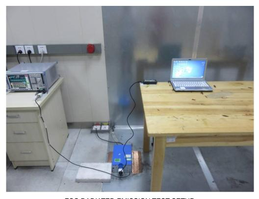
FCC RADIATED EMISSION TEST SETUP
