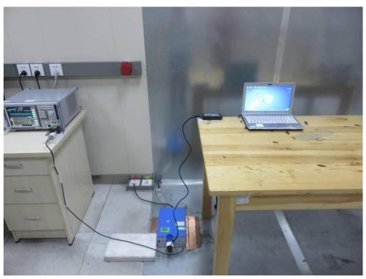
FCC RADIATED EMISSION TEST SETUP
