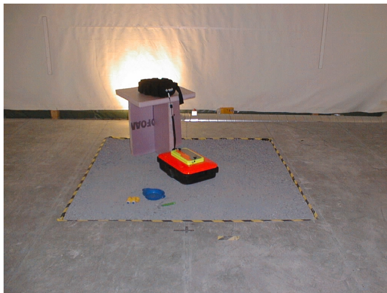
Picture 2: EUT setup on sand bed
