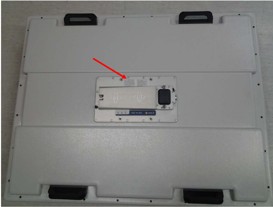
Figure 2. Placement of the FCC labels at the left side of the UWB-unit. Visible at all times.
