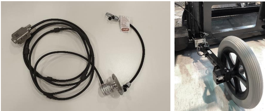
Vehicle mounted encoder and the 300mm measuring wheel
