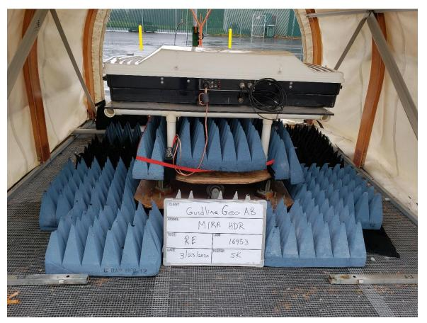
Photograph 2: Radiated Emissions Test Configuration - Back
