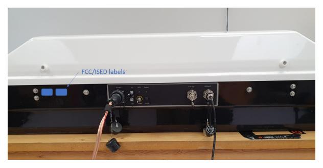
Labels are made of metallized polyester and printed with permanent ink. Printings cannot be removed with commonly used solvents.
