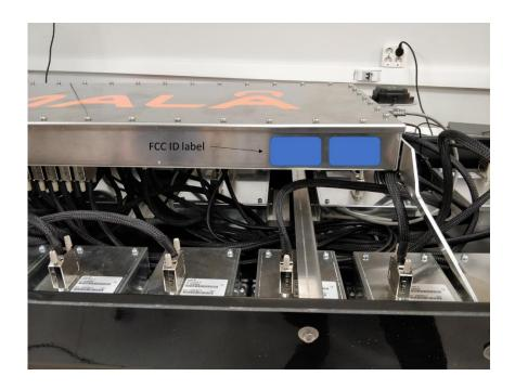
Labels are made of metallized polyester and printed with permanent ink. Printings cannot be removed with commonly used solvents.
