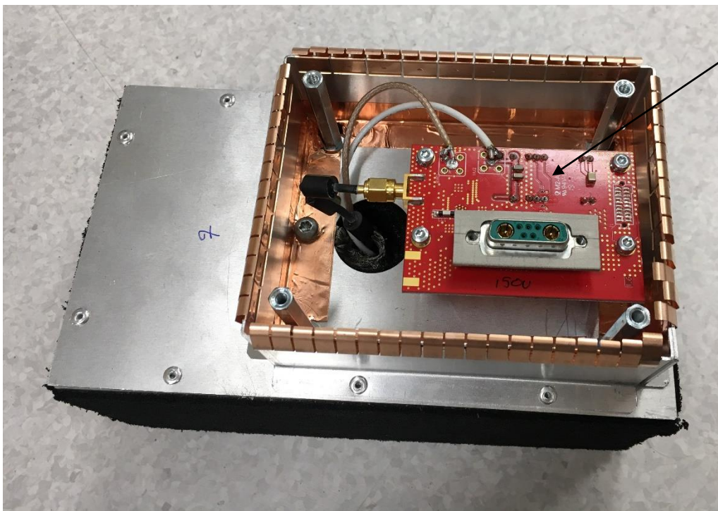
Photo 10: Lid removed, exposing the HV board
