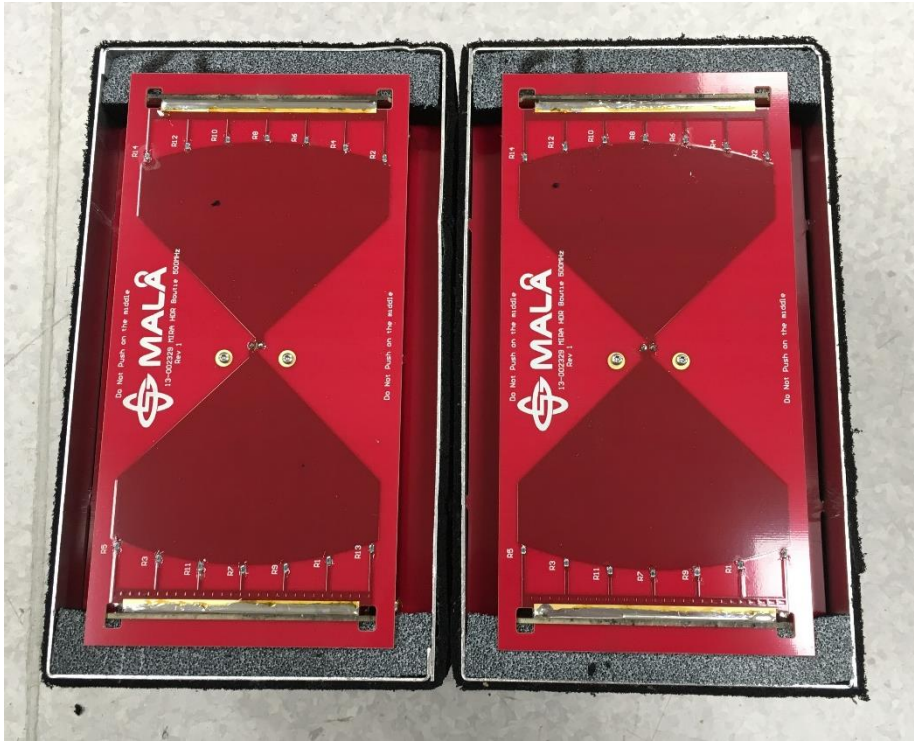
Photo 21: Rx-unit antenna flares
