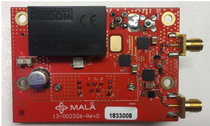
Photo 11, HV board – back
