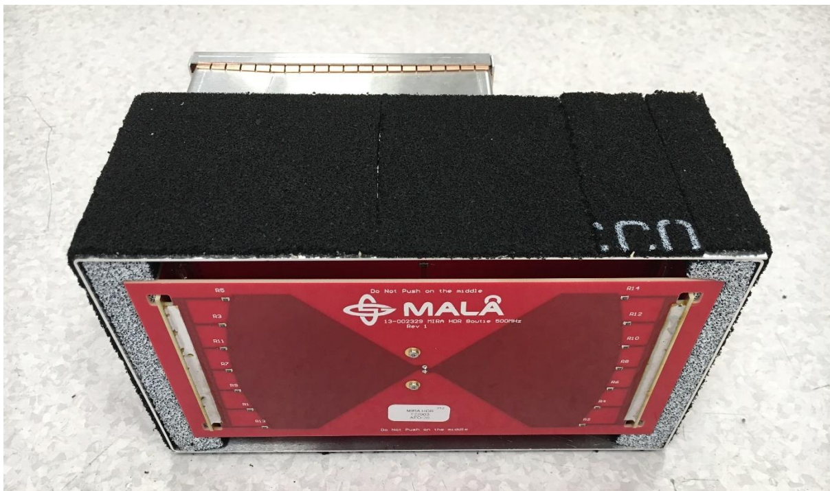
Photo 12: Bottom view of transmitter antenna
