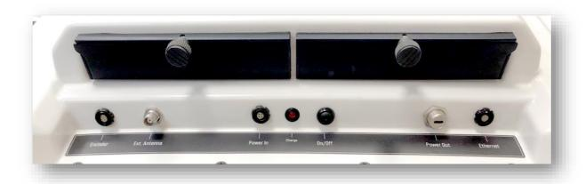
Note: When cables are not connected, the protective caps of the connectors MUST be attached. This prevents dirt and moisture ingress in the connectors.
