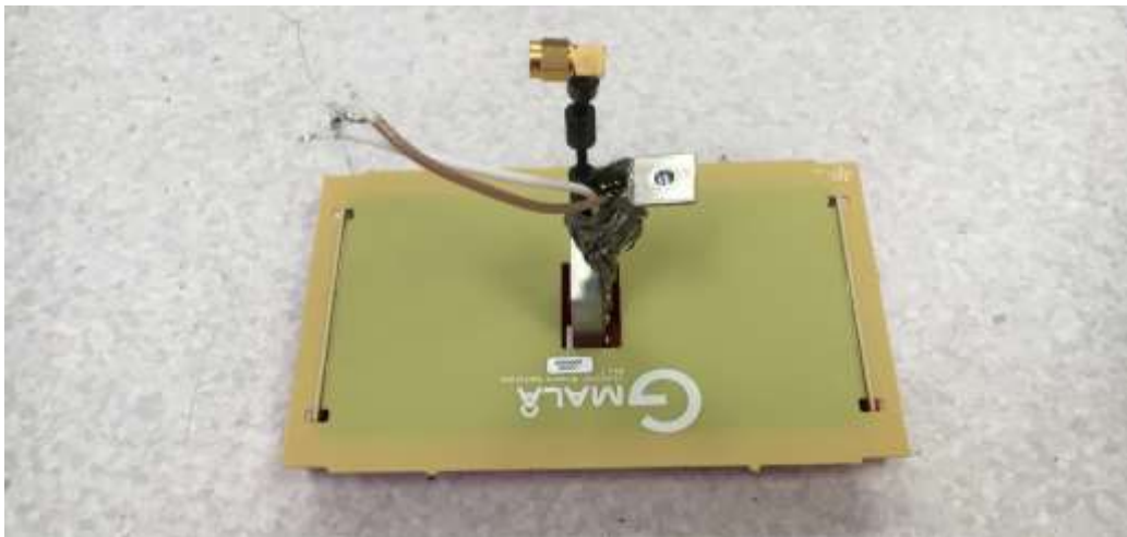
Photo 20: Antenna assembly removed from antenna
