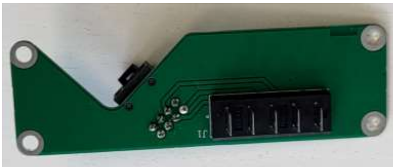
Photo 10: Battery connector board – Back
