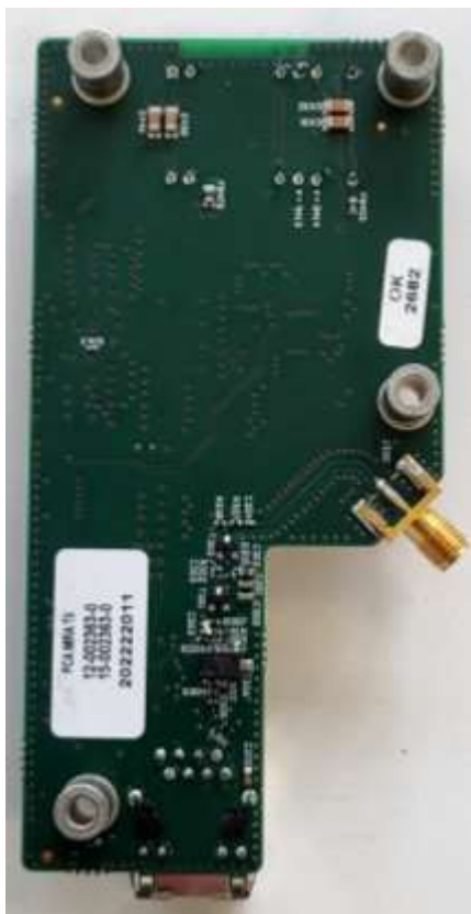
Photo 18, HV board – back
