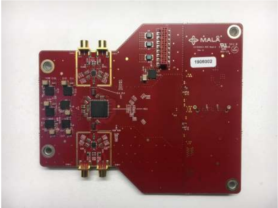
Photo 26: ADC board – front
