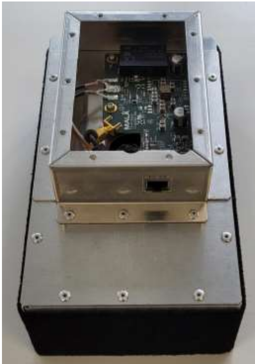
Photo 5: Lid removed, exposing the TX HV board
