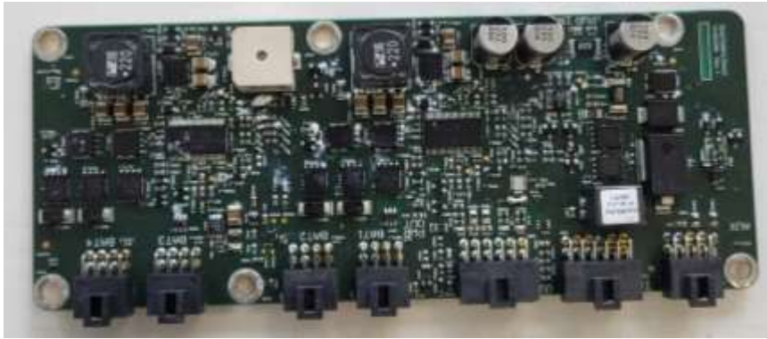
Photo 11: Quad battery board - Front
