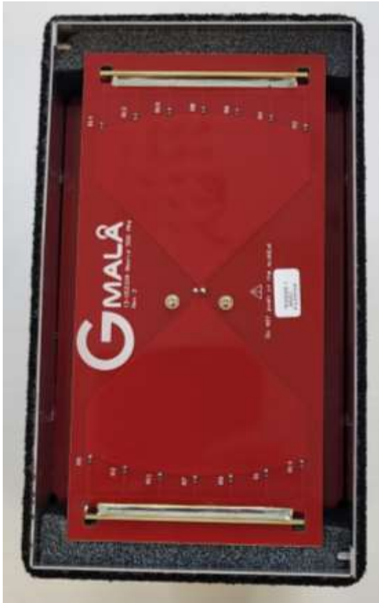
Photo 19: Bottom view of transmitter antenna
