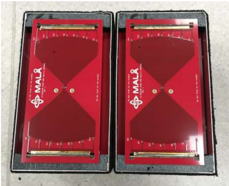
Photo28: Bottom view of transmitter antenna
